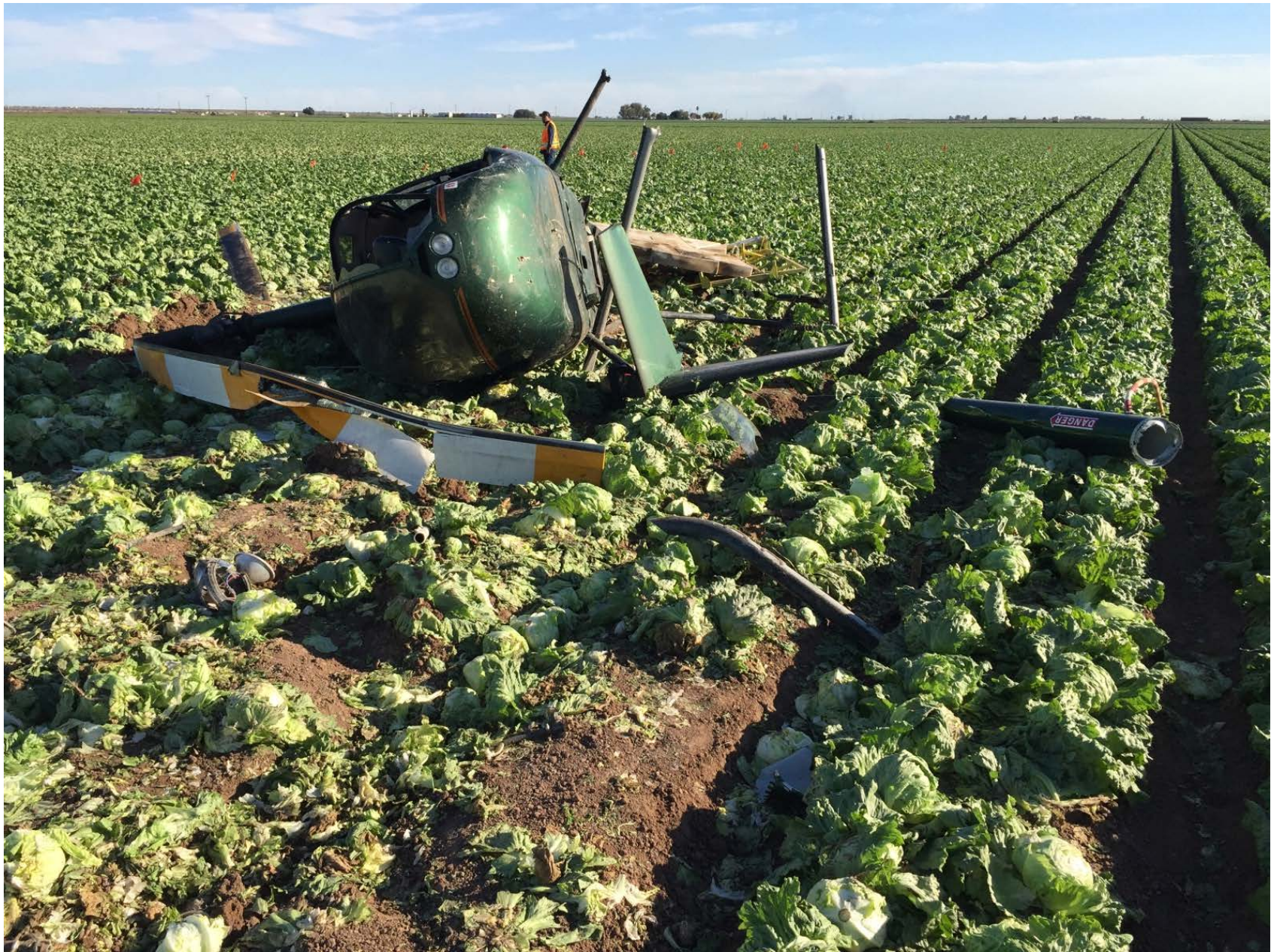
Photo 1 – View of the damage to both rotor drive systems (Courtesy of FAA)
