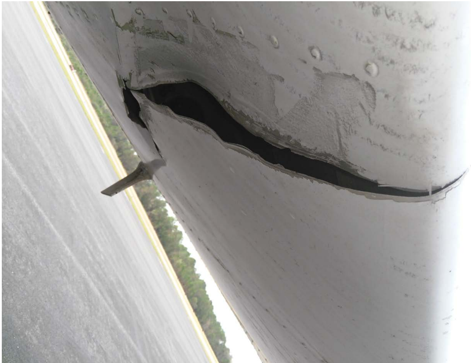
Photo 1 – View of damaged left wing (photo courtesy of the FAA)
