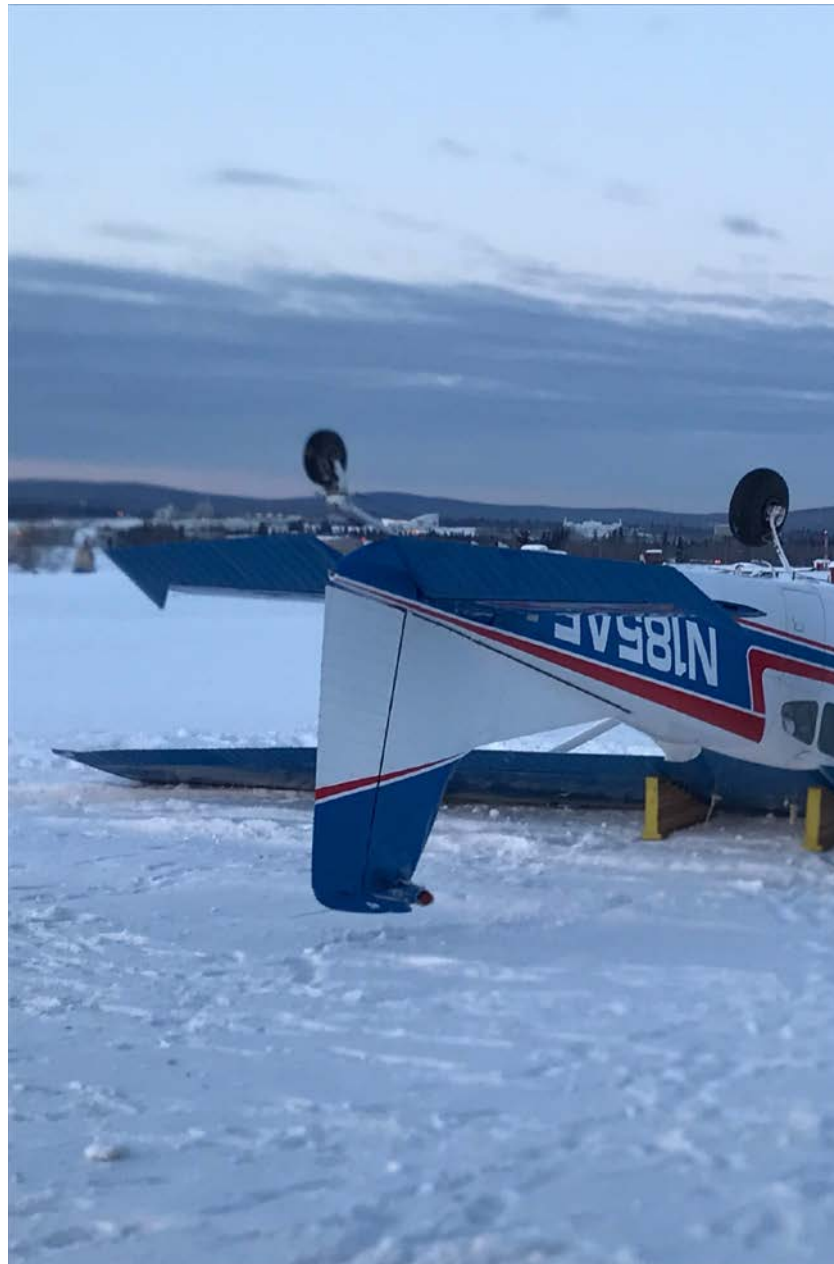
Photo 1 –Substantially Damaged Vertical Stabilizer (Photo Courtesy of FAA)
