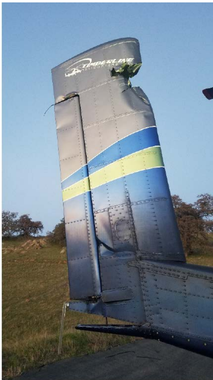
Photo 3 – View of damage to the vertical stabilizer (Courtesy of Operator)
