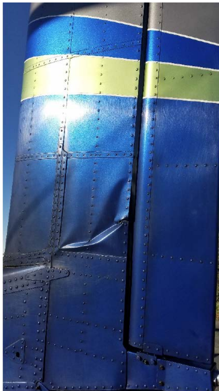
Photo 3 – View of damage to the vertical stabilizer (Courtesy of Operator)
