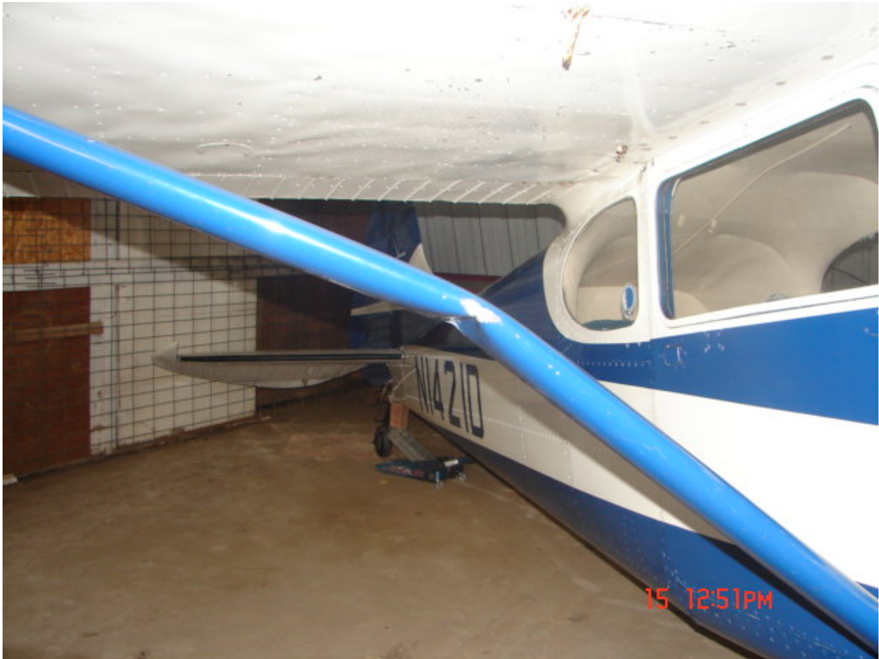
Photo 1 – View of damaged right wing lift strut (photo courtesy unknown)
