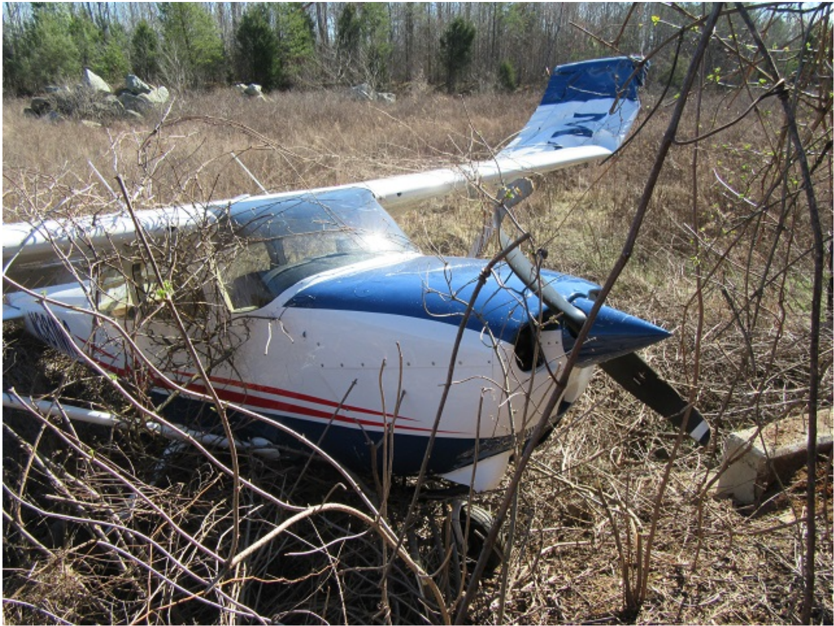
Photo 1 – Airplane with Substantially Damaged Left Wing (Photo Courtesy of FAA)
