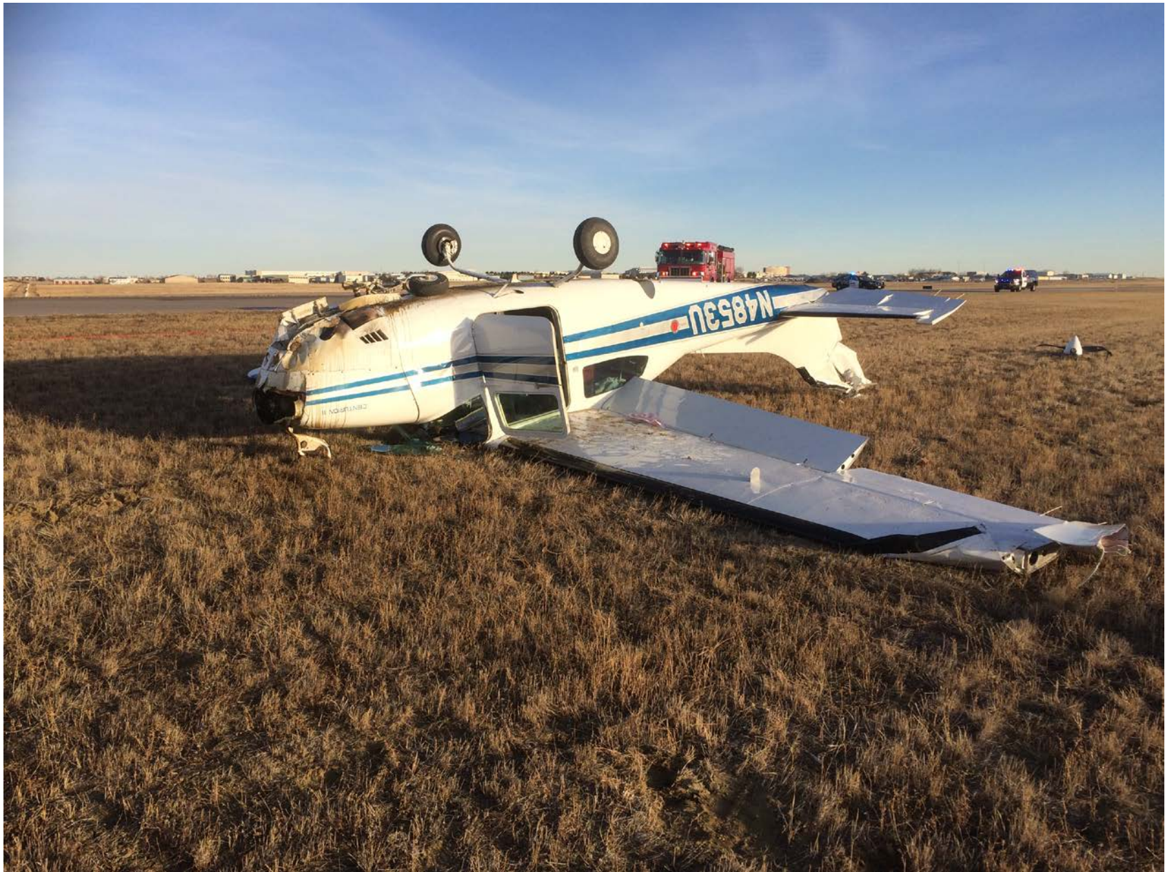
Photo 1 – Airplane Nosed Over to the Left of the Landing Runway (Photo Courtesy of FAA)
