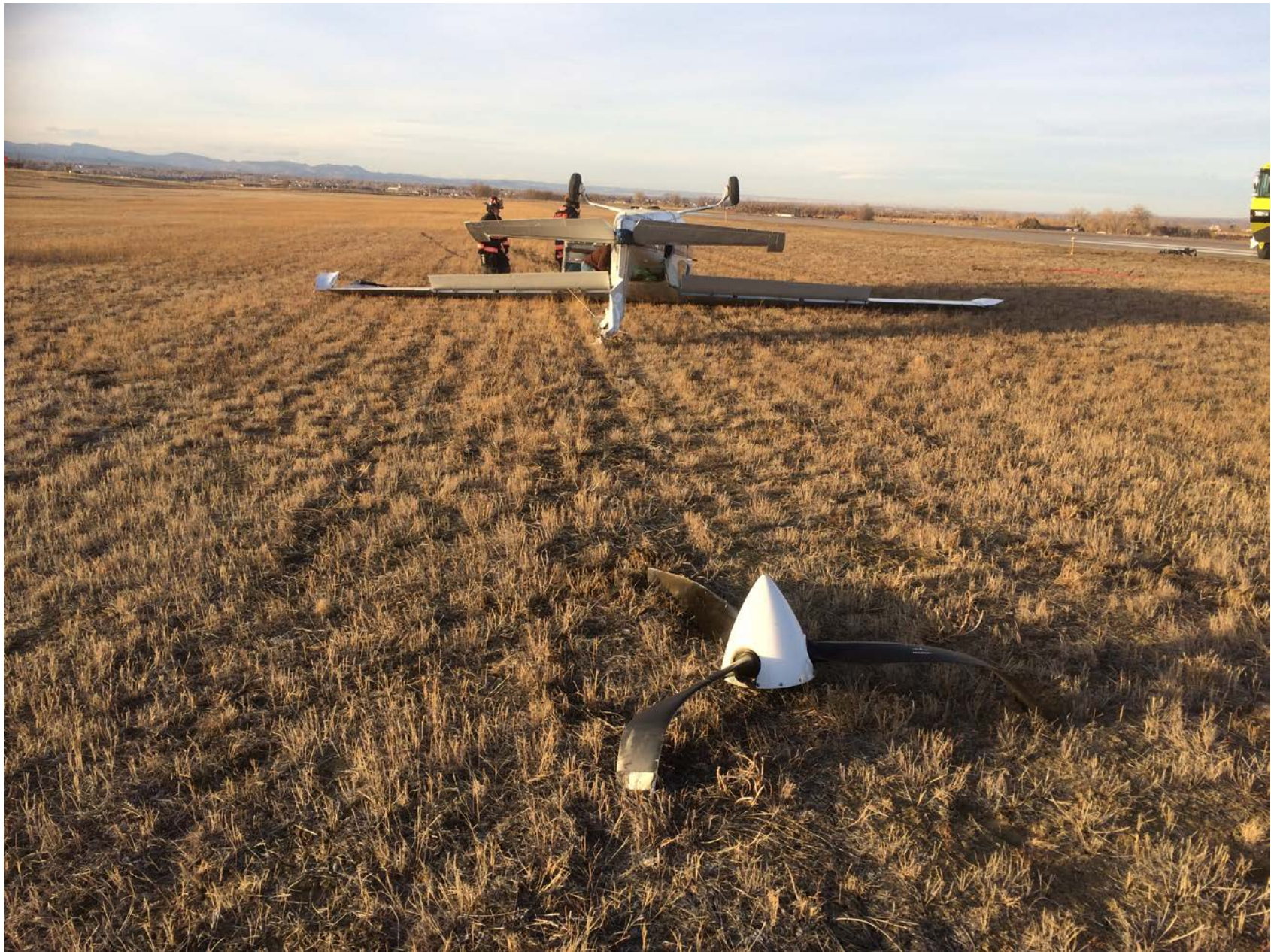
Photo 2 – Propeller Separated from the Main Wreckage (Photo Courtesy of FAA)
