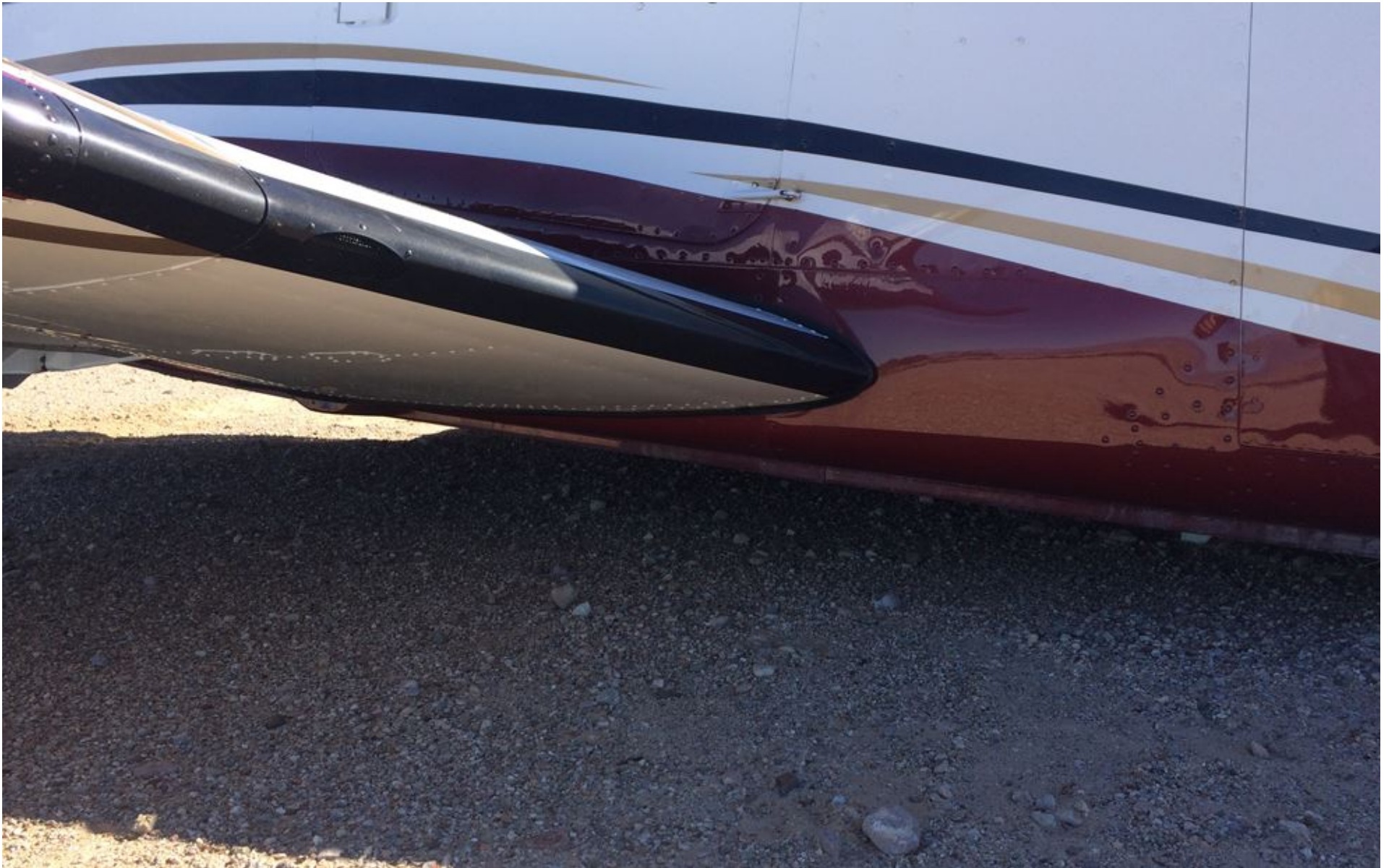
Photo 1 – Damaged Fuselage and Wing Attach Point (Photo Courtesy of FAA)
