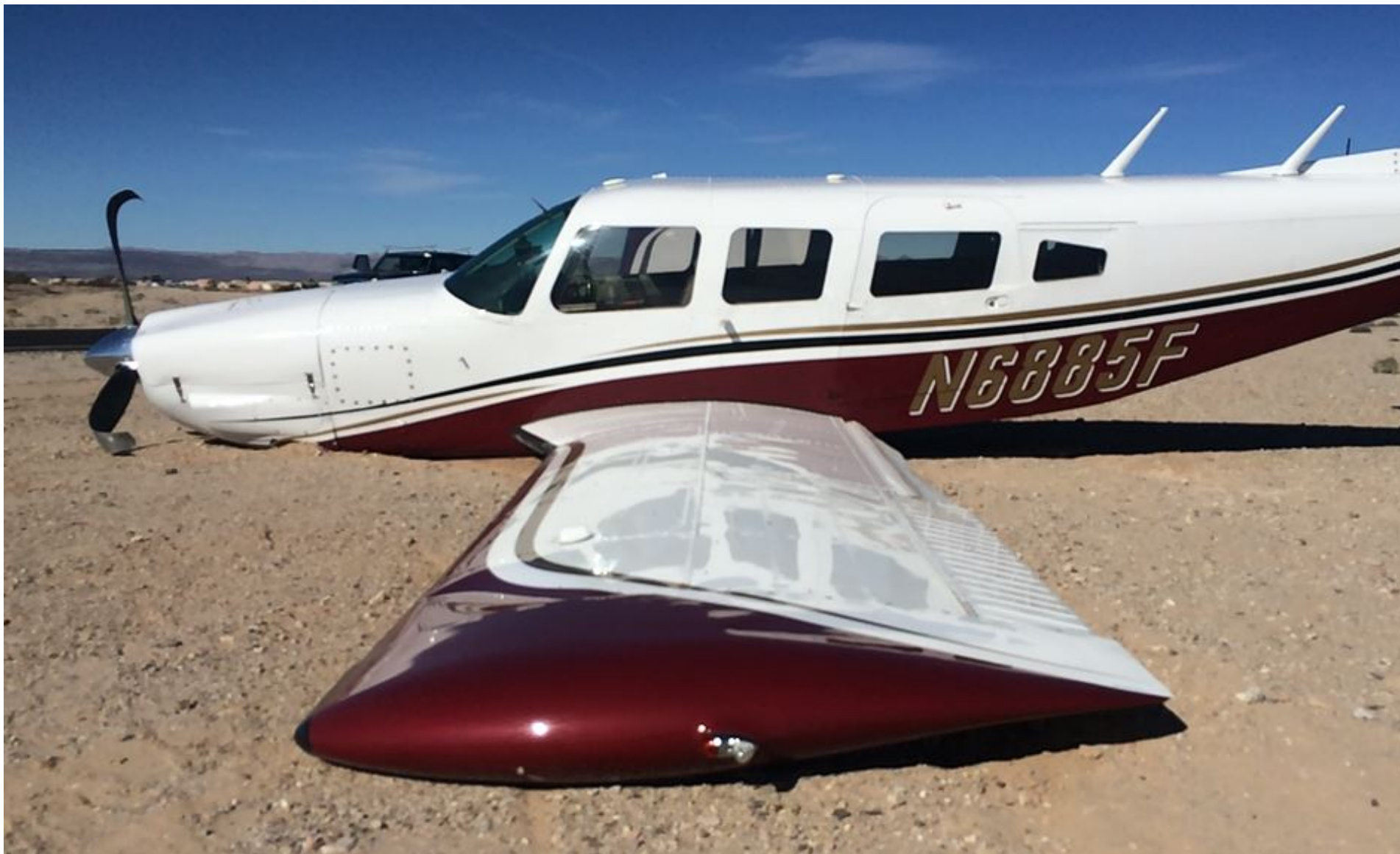
Photo 2 – Damaged Left Wing and Collapsed Landing Gear (Photo Courtesy of FAA)
