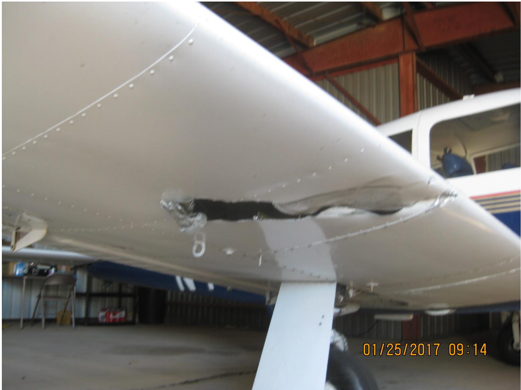
Photo 1 – View of substantial damage to the right wing (photo courtesy of the FAA)
