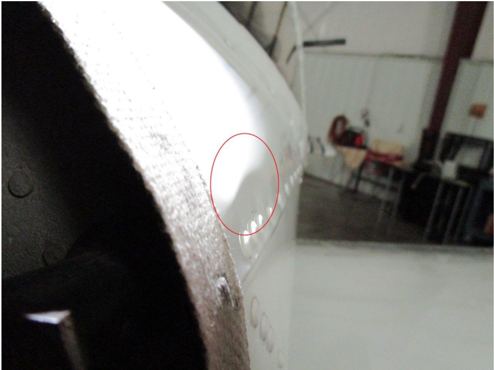
Photo 2 – Buckled Skin Along Fuselage (Photo Courtesy of FAA)
