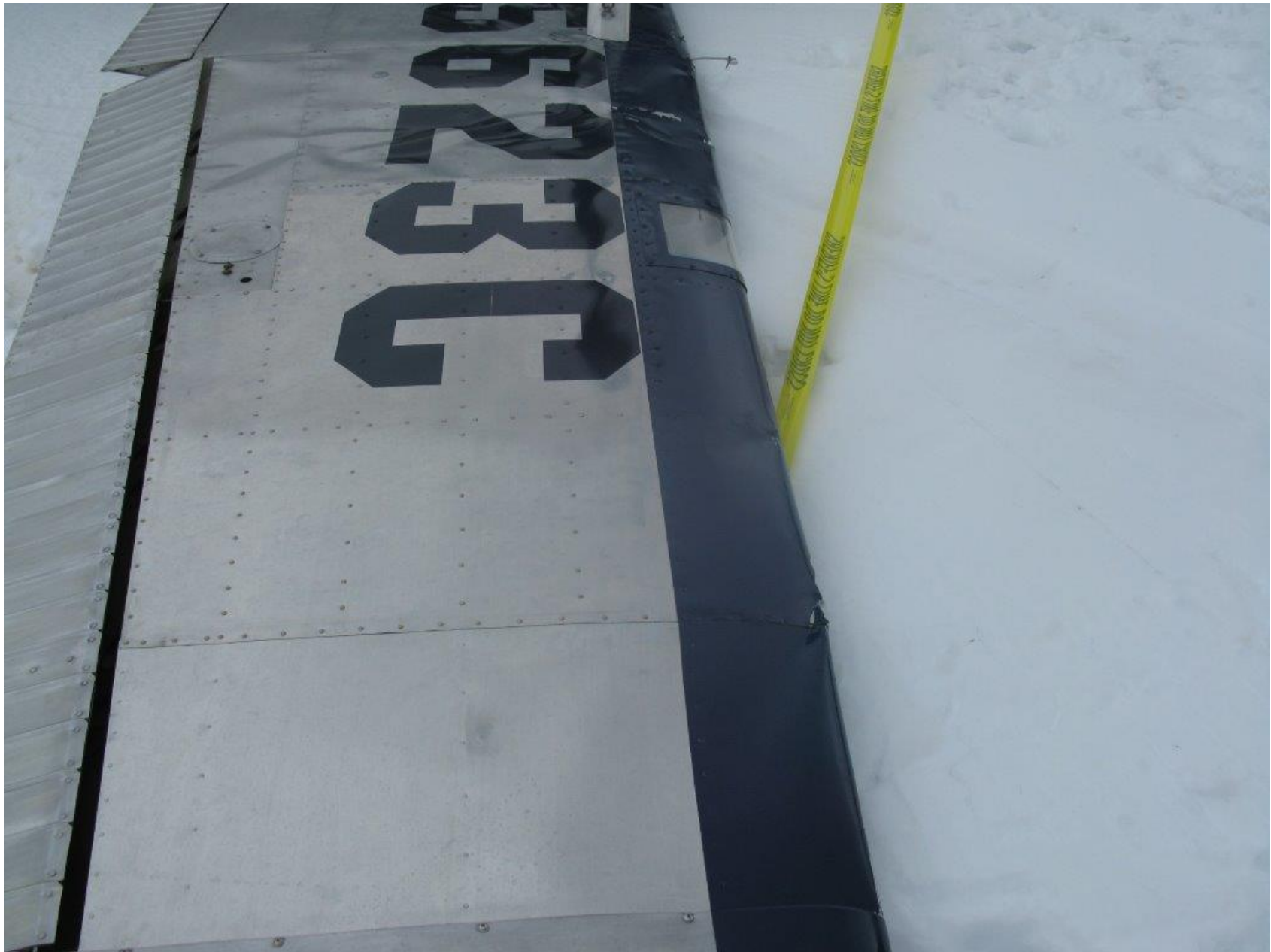
Photo 1 – View of substantial damage to left wing (Courtesy of FAA)
