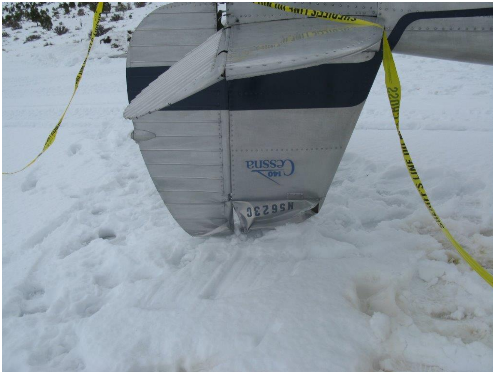
Photo 2 – View of substantial damage to horizontal stabilizer and rudder (Courtesy of FAA)
