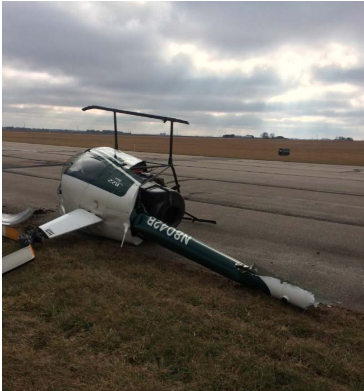
Photo 1 – View of damaged helicopter tail boom (photo courtesy of the flight instructor)
