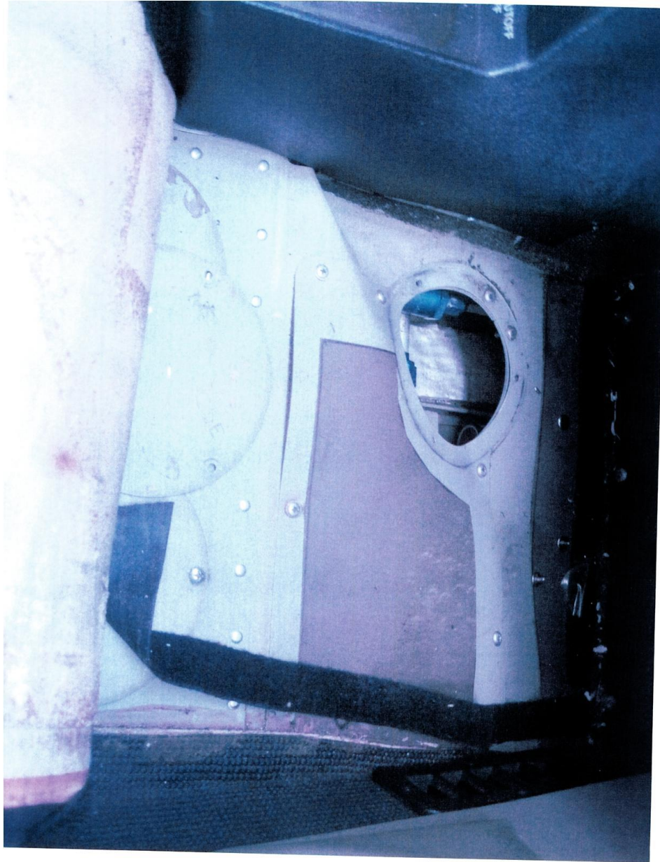
Photo 2 – View of damaged interior floorboard (Photo courtesy of the FAA)
