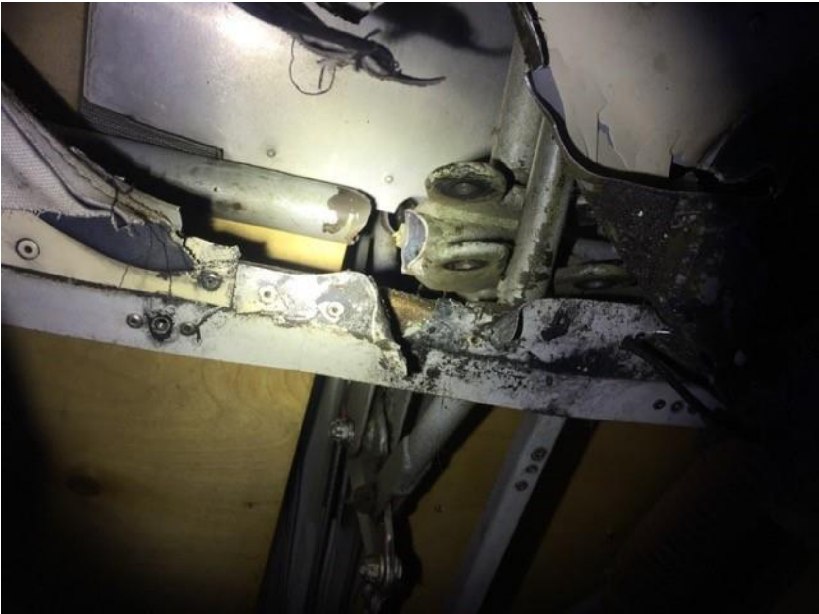
Photo 1 – View of broken tubing near landing gear (photo courtesy of the FAA).
