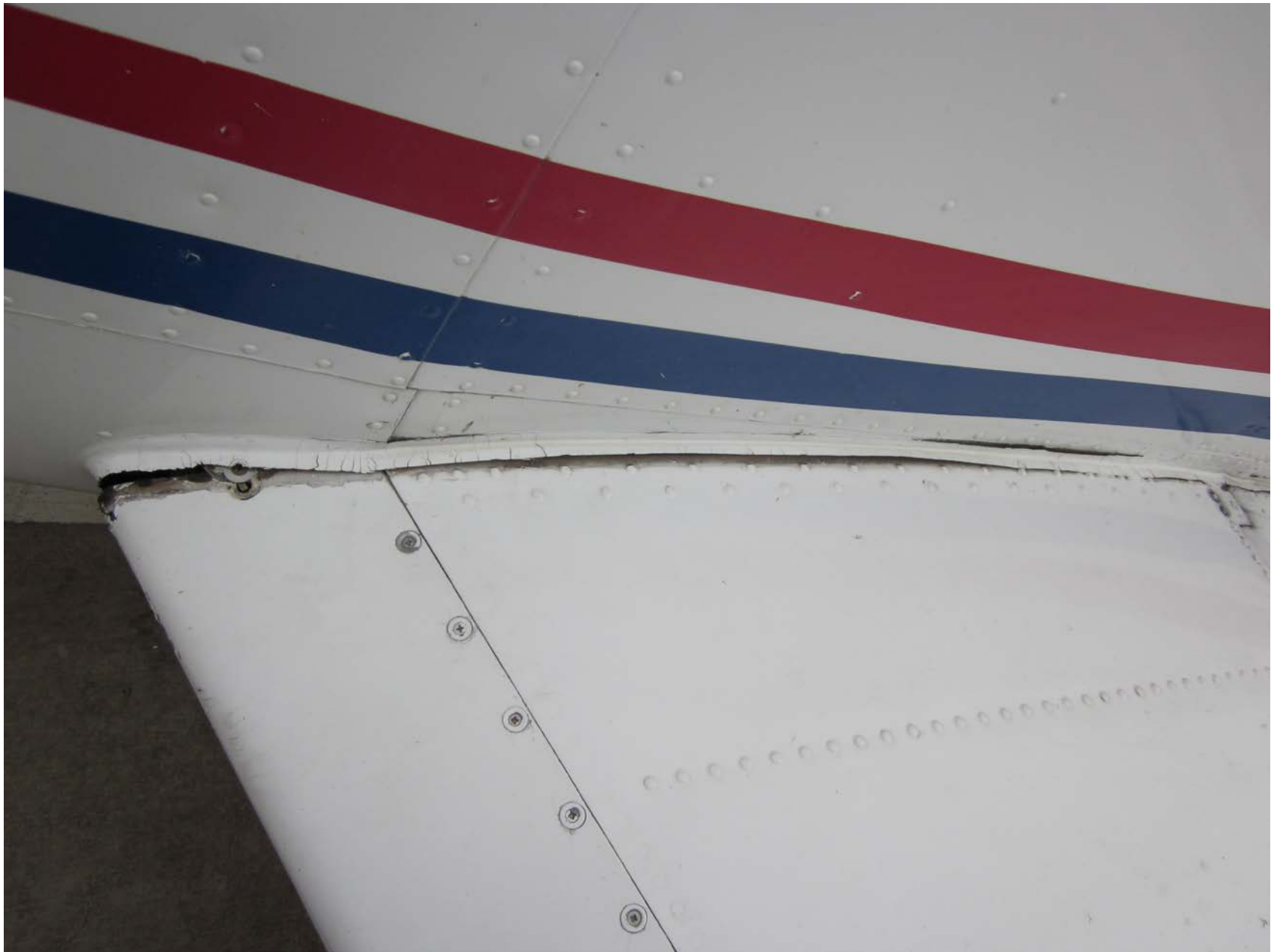
Photo 2 – View of damage to left wing root (Courtesy of FAA)
