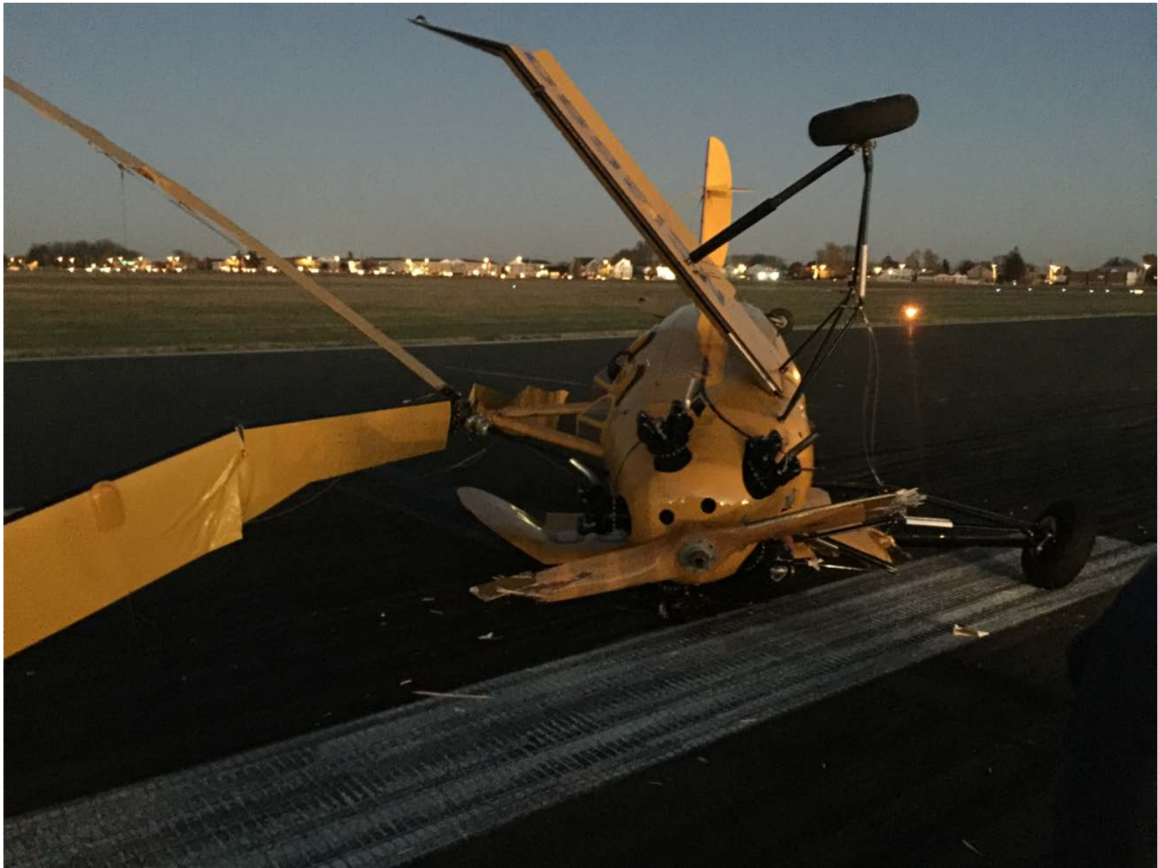
Photo 1 – View of damage to the right wing and main rotor system (Courtesy of FAA)
