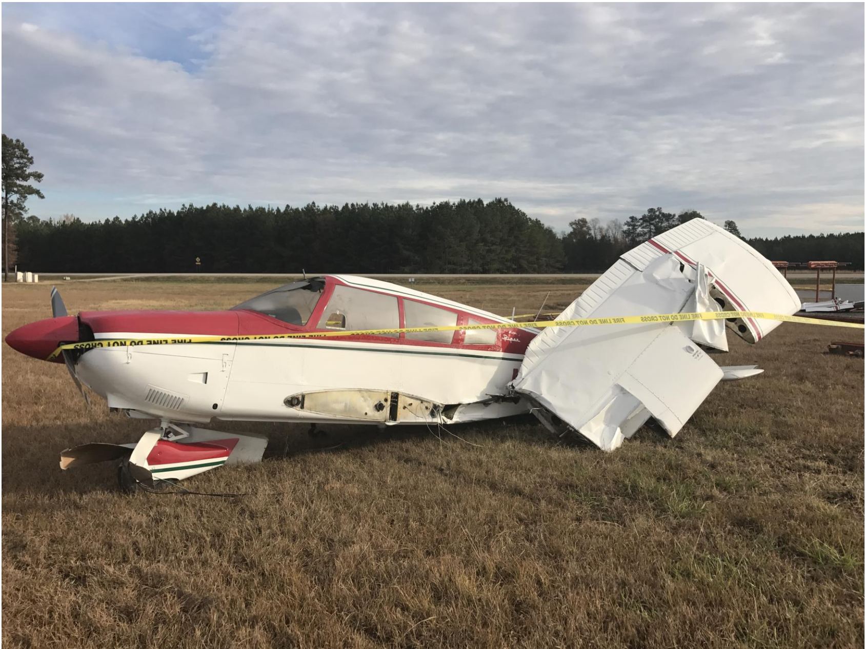
Photo 1 – View of substantial damage to both wings (photo courtesy of the FAA).
