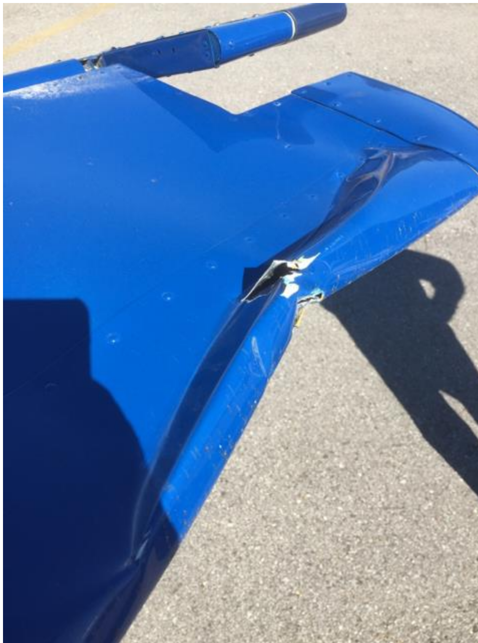
Photo 1 – View of damaged left horizontal stabilizer (photo courtesy of flight club manager)
