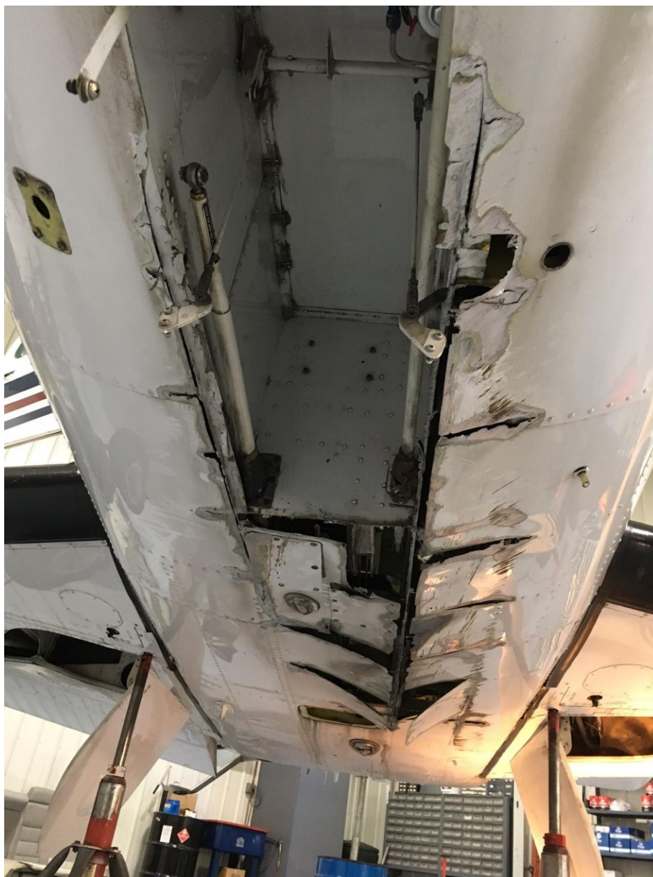
Photo 1 – View of damaged fuselage (photo courtesy unknown)
