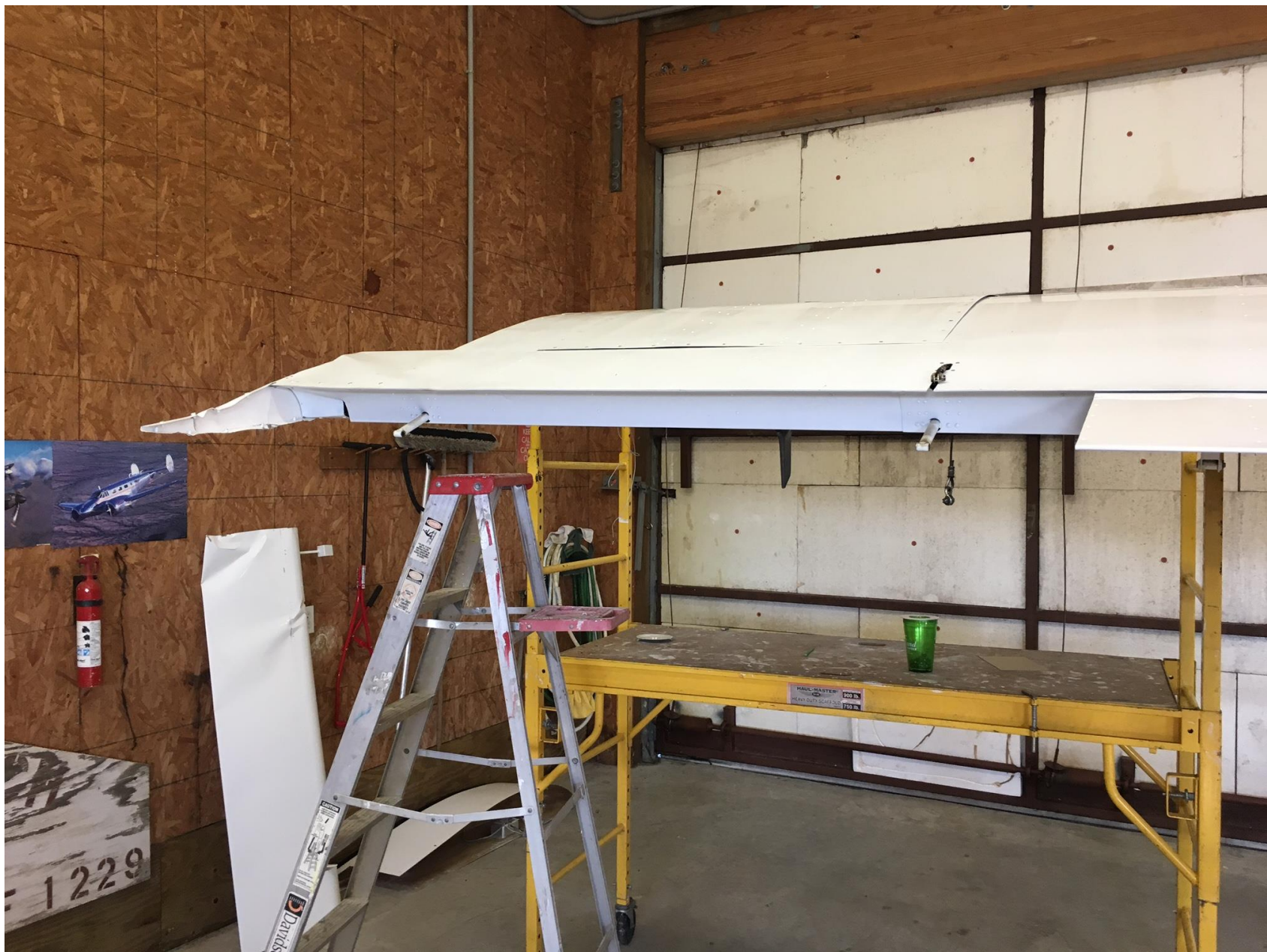
Photo 1 – Rear view of damaged left wing and aileron (Photo courtesy of pilot)
