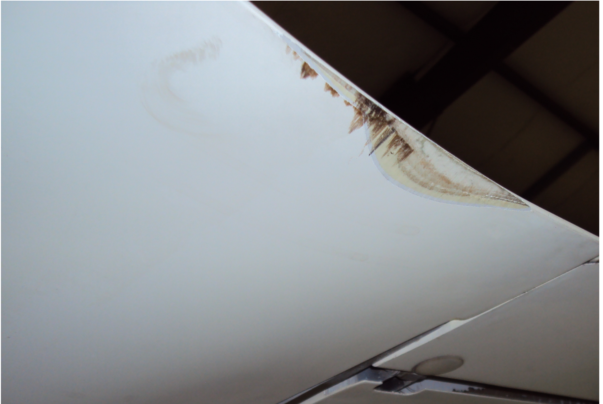
Photo 3 – View of damage to the trailing edge of the outboard left wing (Courtesy of FAA)
