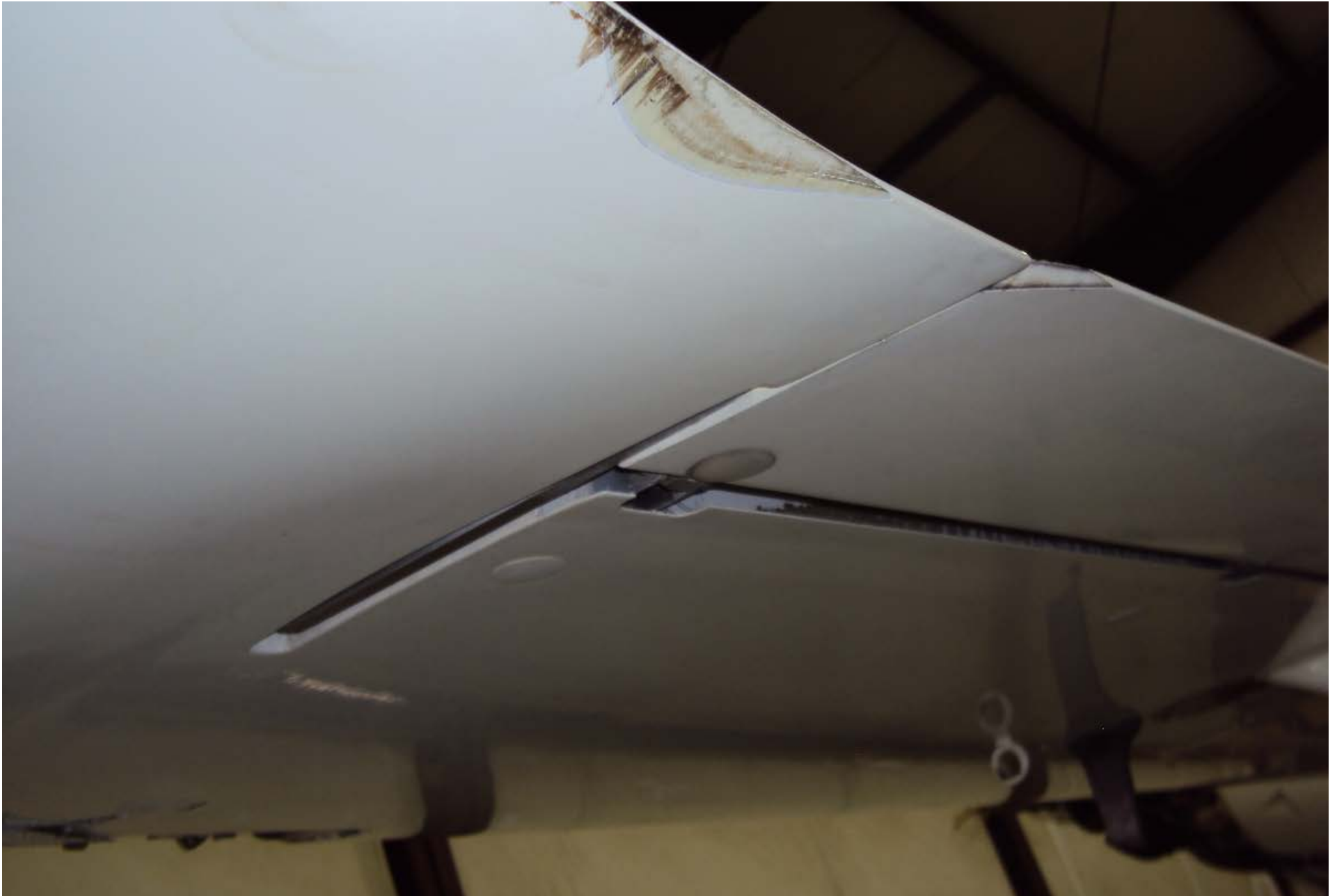
Photo 4 – View of damage to left aileron (Courtesy of FAA)
