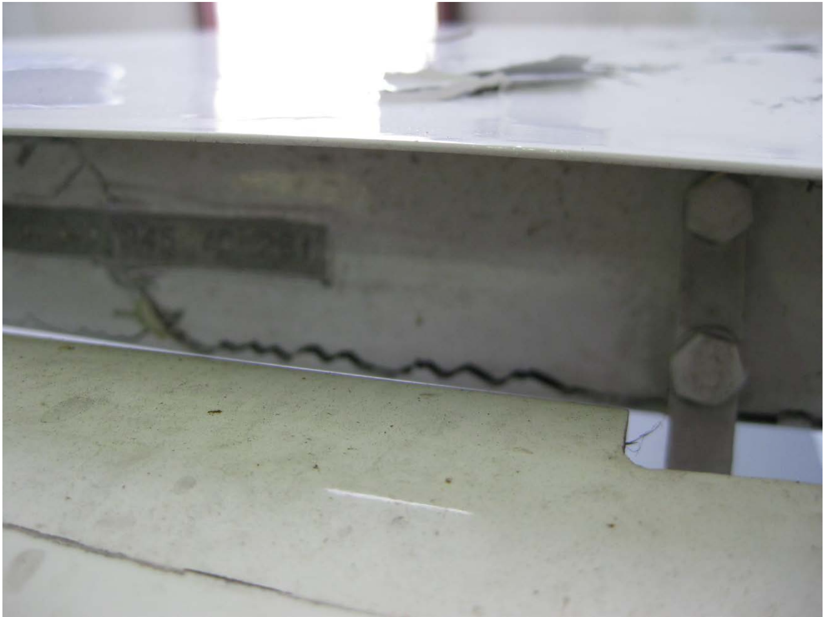
Photo 2 – View of substantial damage to the composite left wing (Courtesy of FAA)
