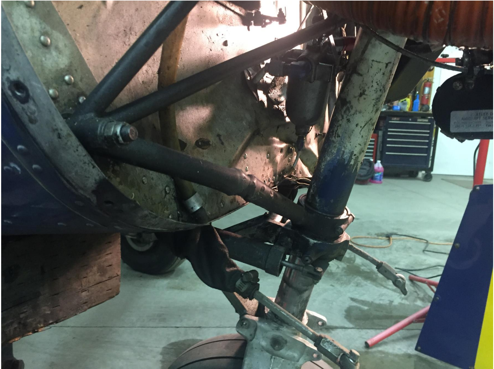
Photo 1 – View of damaged firewall (photo courtesy of the flight instructor)
