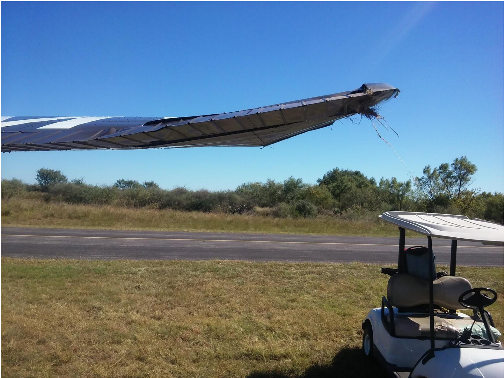
Photo 2 – Rear view of damaged right wing and aileron (Photo courtesy of the FAA)
