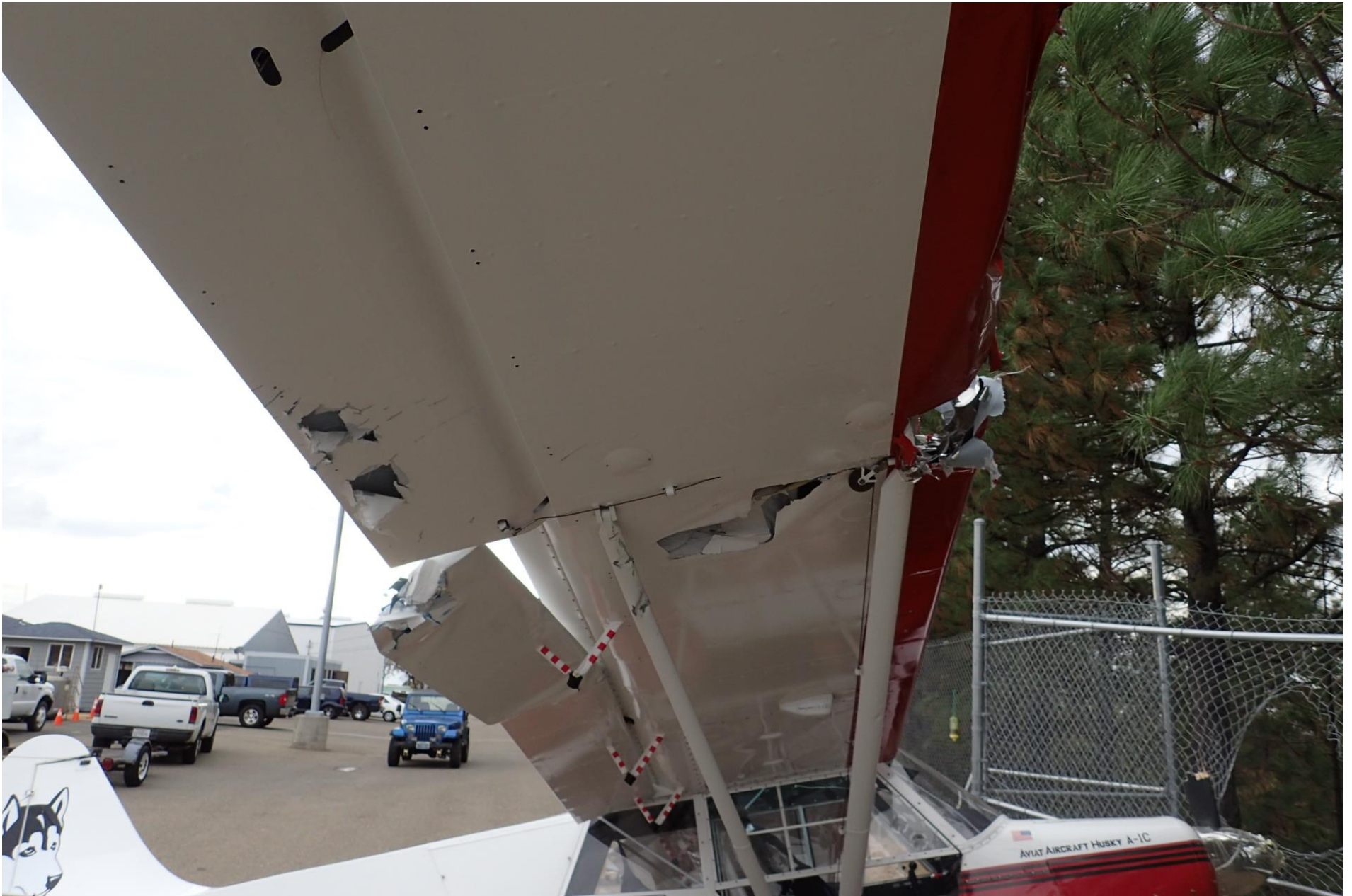
Photo 2 - View of damaged right wing and aileron (Photo courtesy of the FAA)
