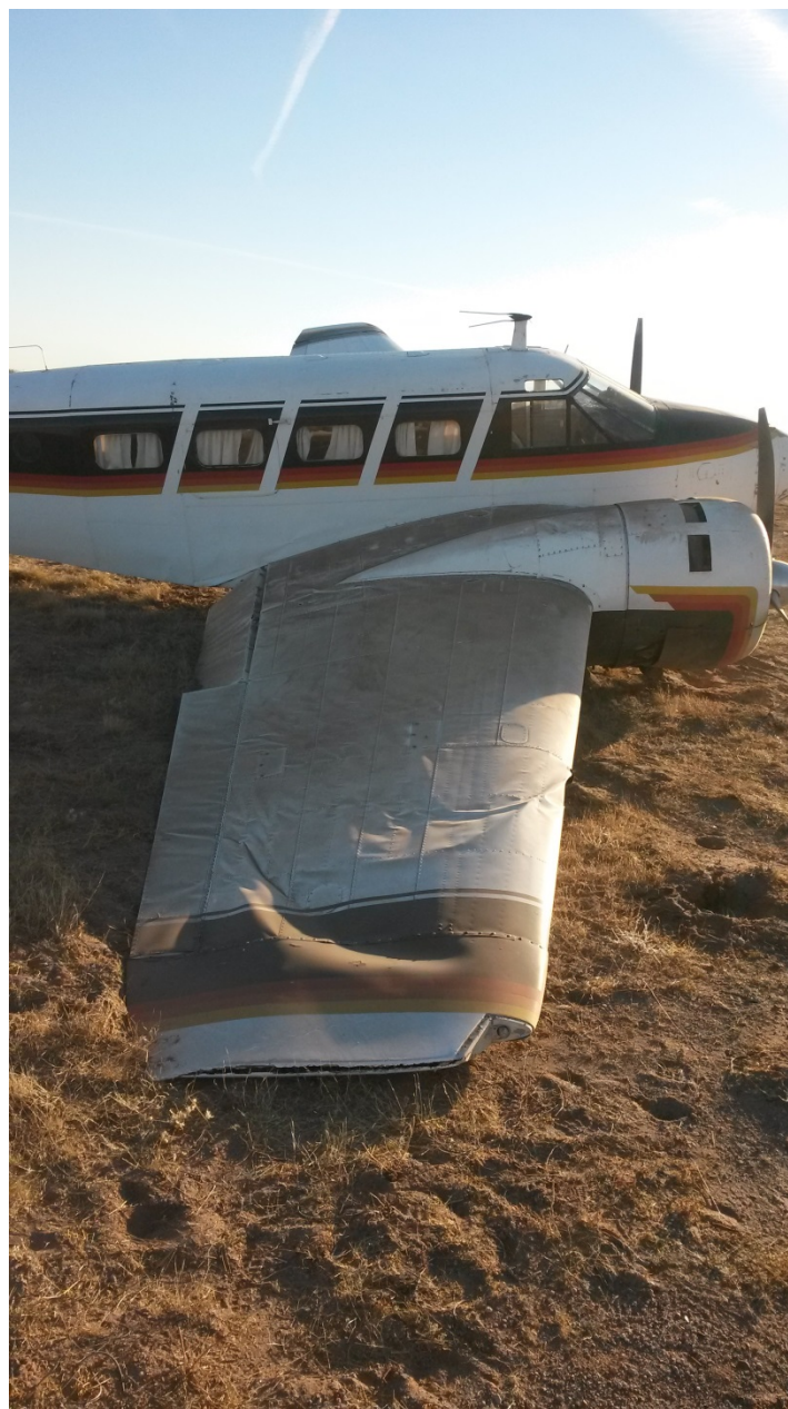
Photo 1 – Substantially Damaged Right Wing (Photo Courtesy of FAA)
