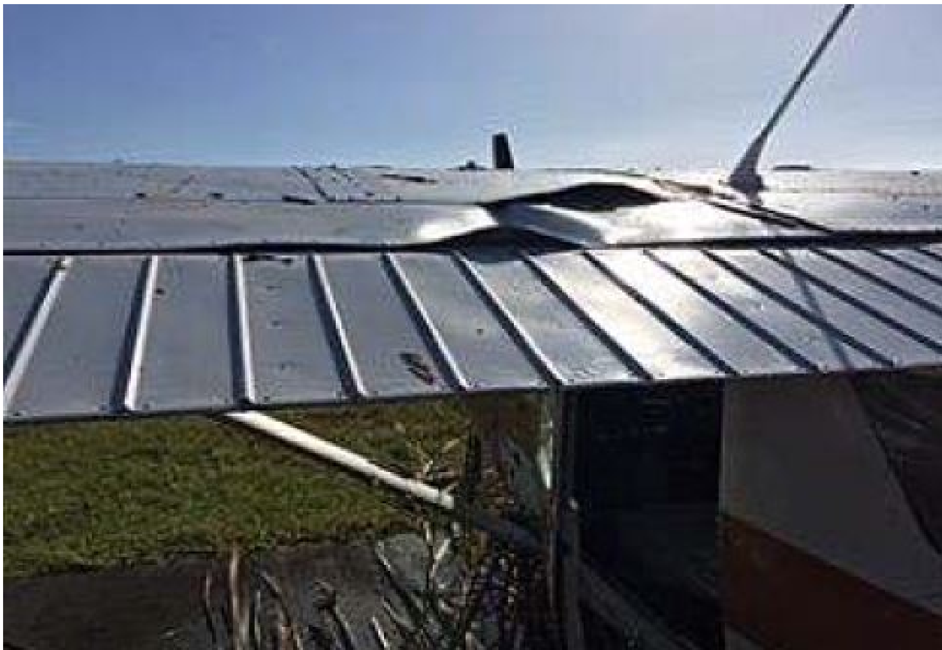
Photo 1 – Substantially Damaged Left Wing (Photo Courtesy of FAA)
