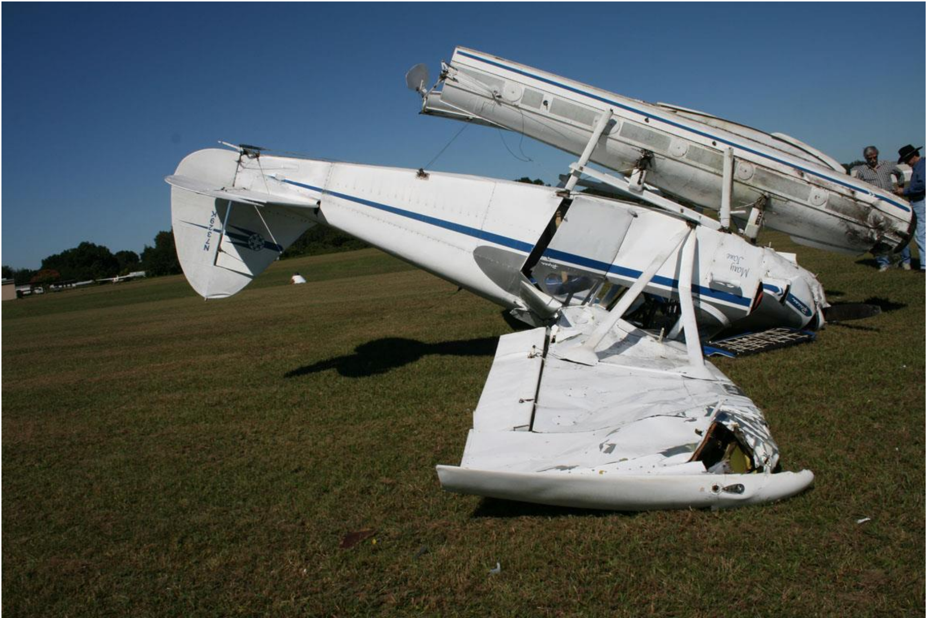
Photo 1 – View of damaged airplane inverted on the runway (Photo courtesy of the FAA)
