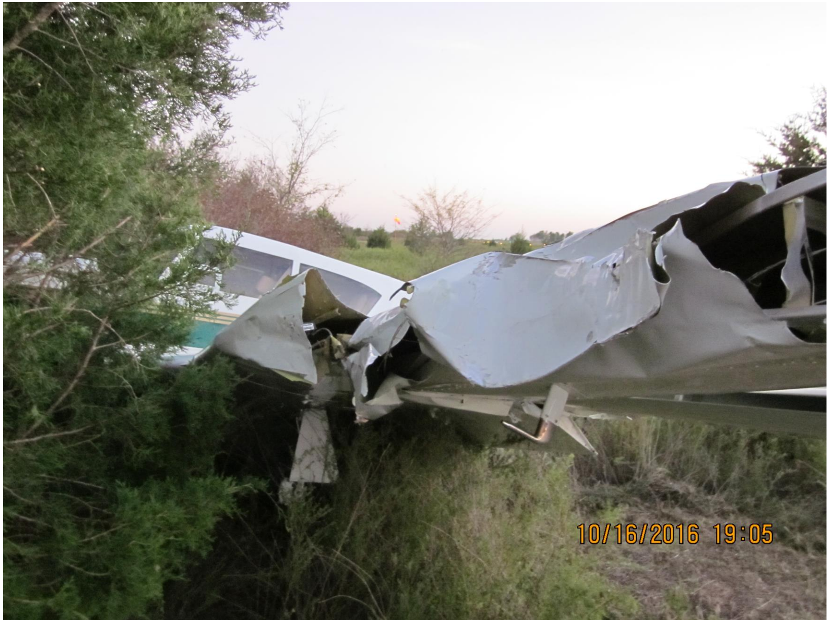
Photo 2 - Front view of damaged left wing (Photo courtesy of the FAA)
