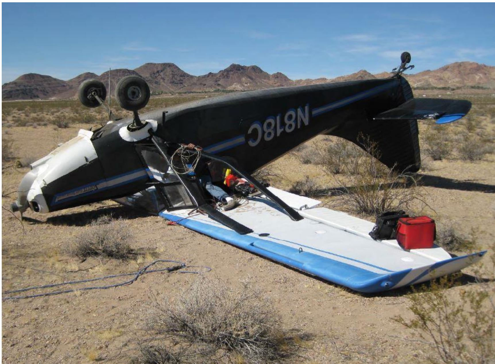
Photo 1 – View of the right wing strut damage (photo courtesy of the FAA)
