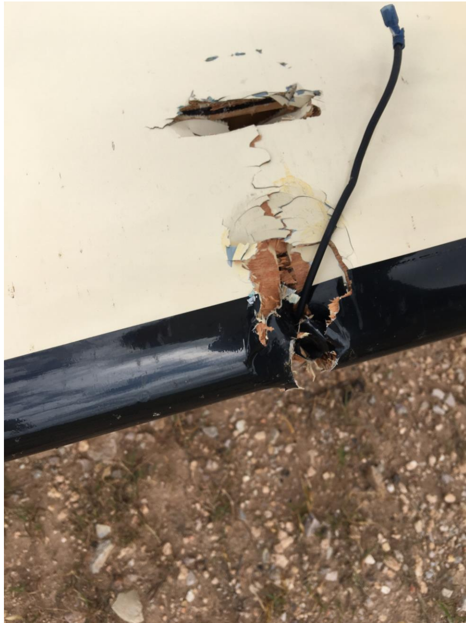
Photo 2 - View of the left wing damage (photo courtesy of the FAA)
