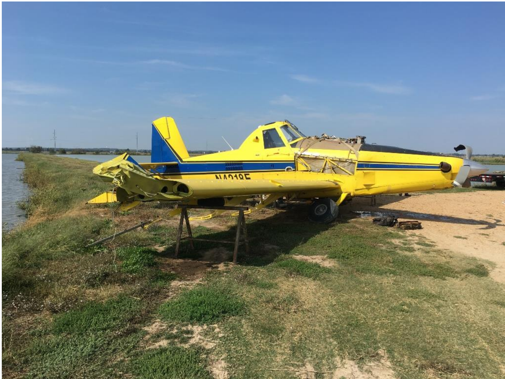
Photo 1 – View of damaged right wing (photo courtesy of recovery company)
