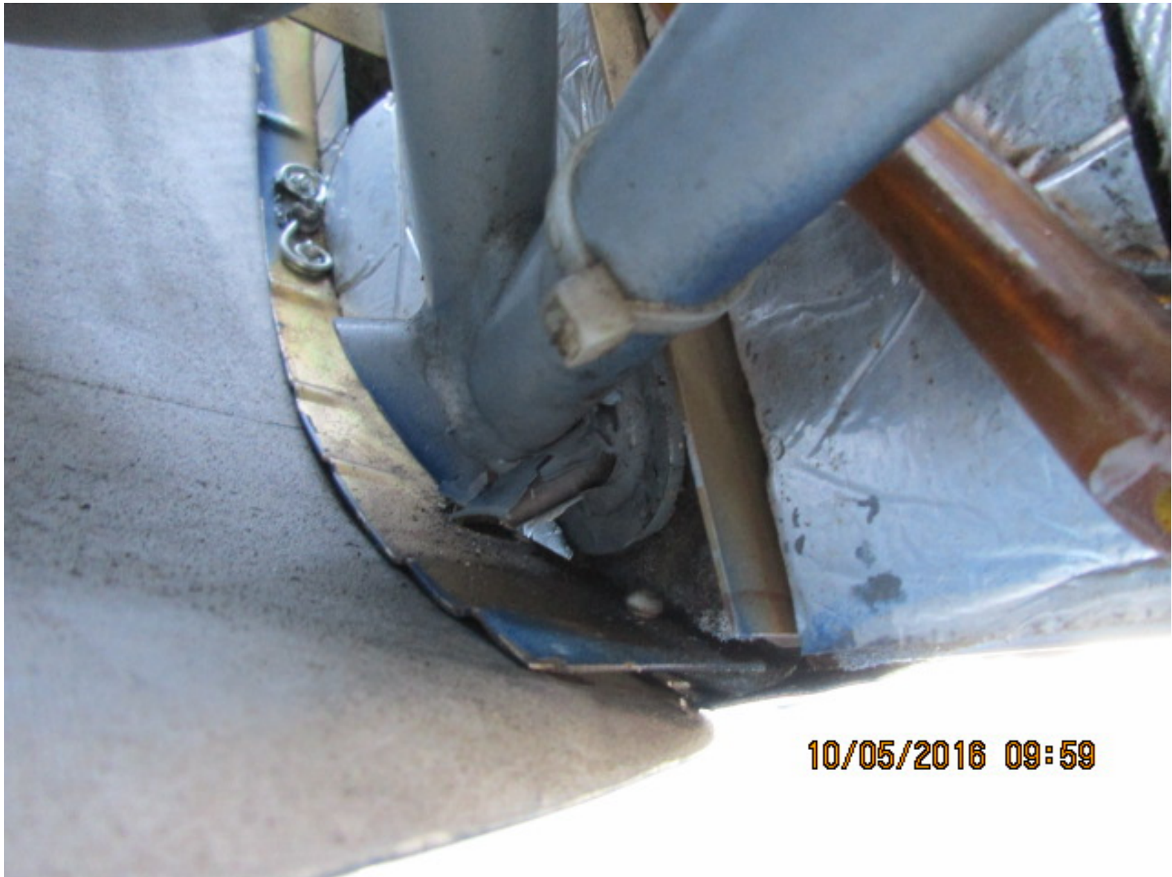
Photo 1 – Damaged Engine Mount (Photo Courtesy of FAA)
