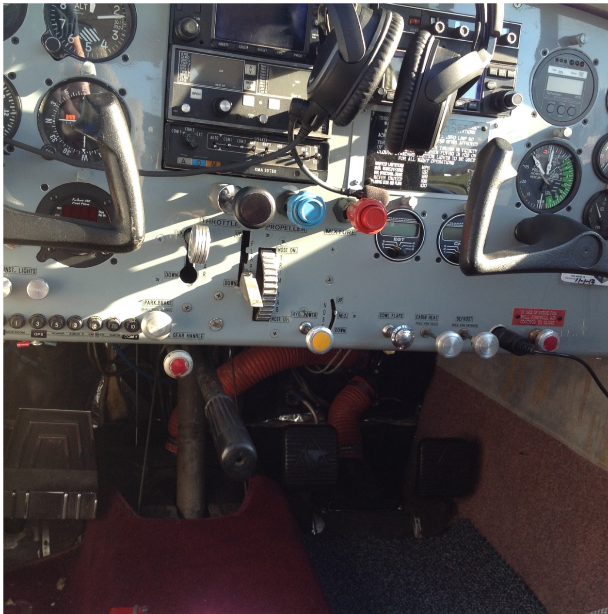
Photo 3 – Landing Gear Handle in the UP Position (Photo Courtesy of FAA)
