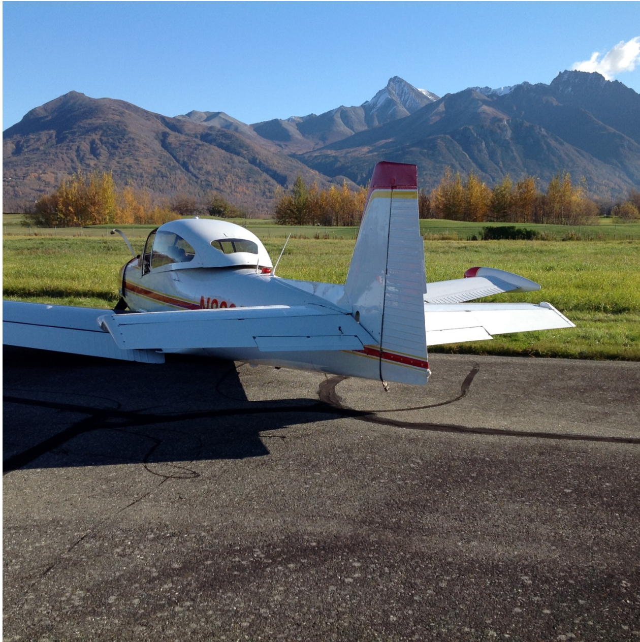
Photo 1 – Airplane on Runway with Landing Gear Retracted (Photo Courtesy of FAA)
