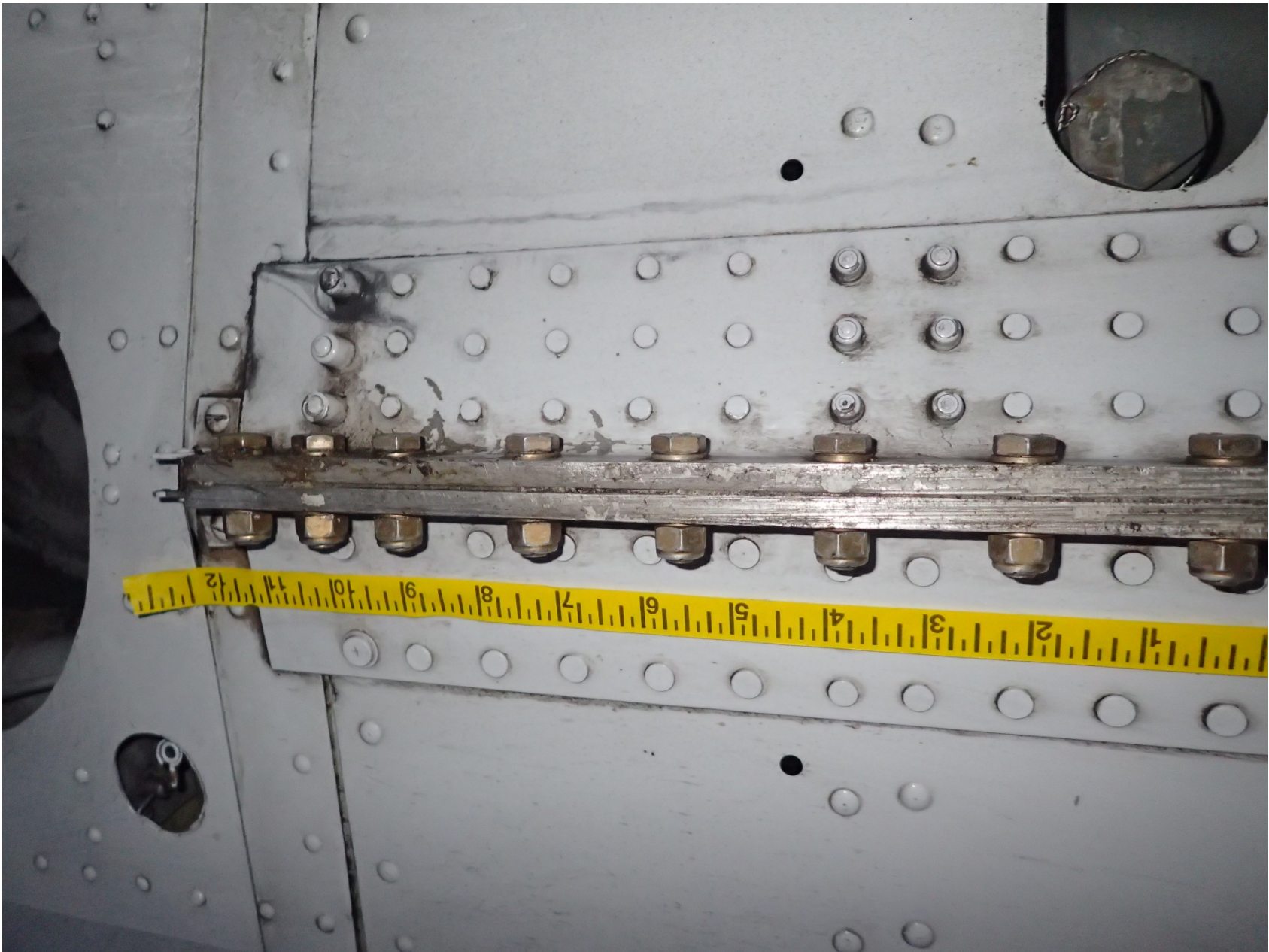
Photo 2 – Damage to Underside of the Fuselage (Photo Courtesy of FAA)
