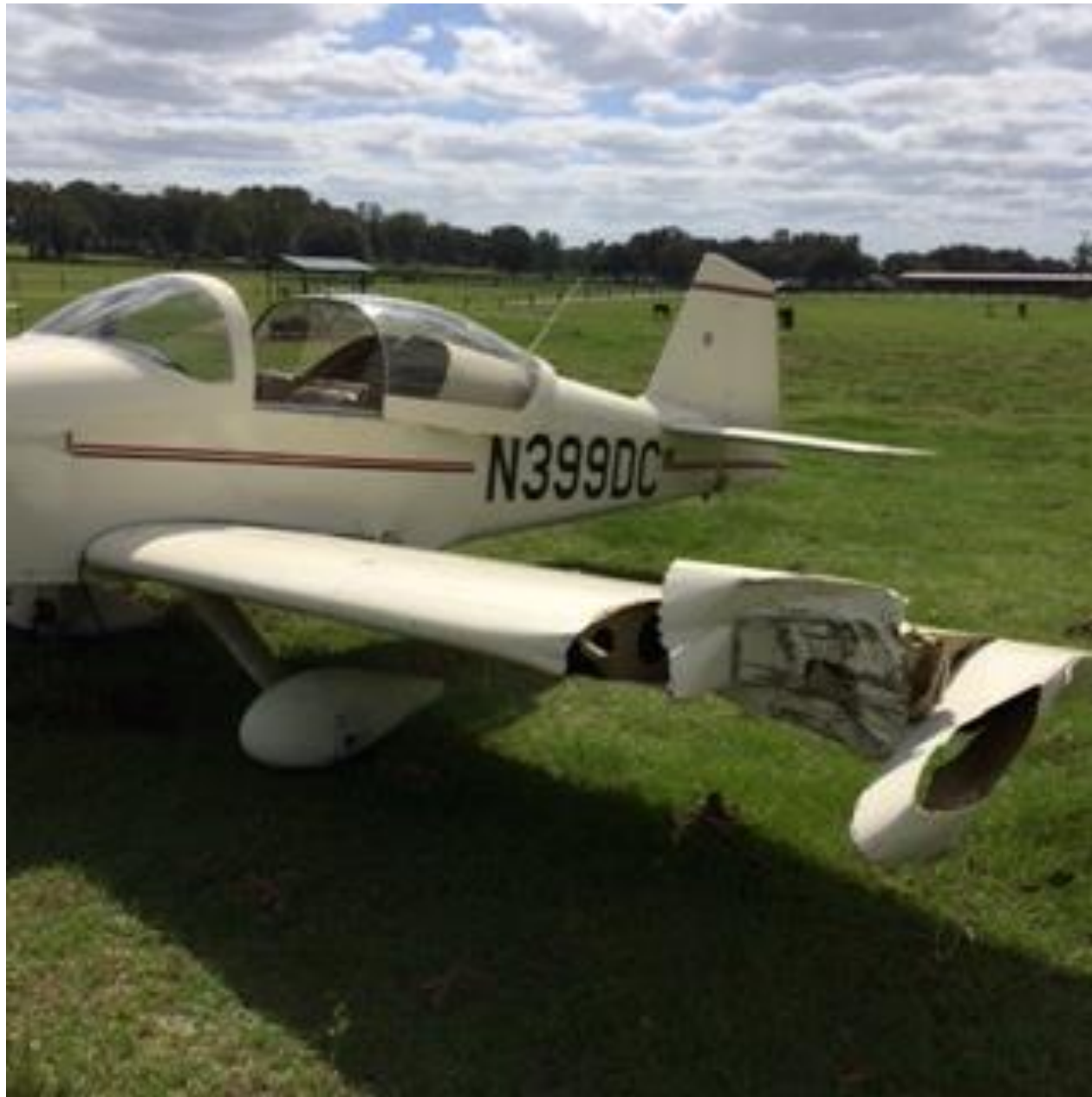
Photo 1 – Damage to the left wing (Photo courtesy of the FAA)
