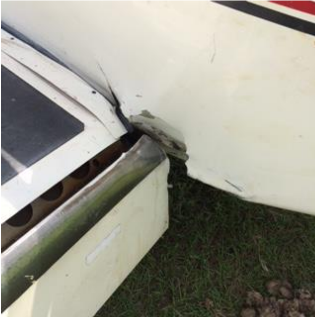
Photo 2 – Damage to the left wing and fuselage (Photo courtesy of the FAA)
