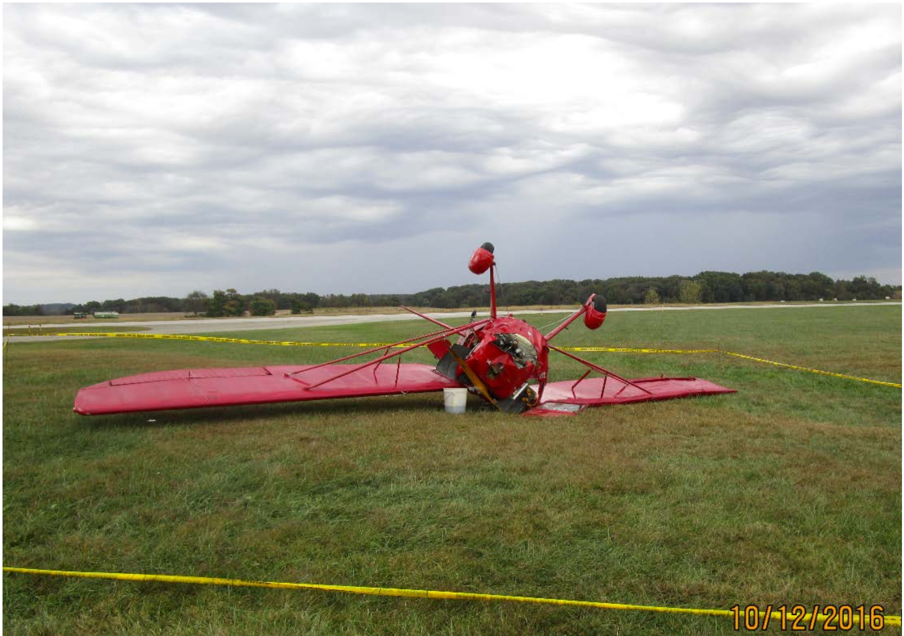
Photo 1 – View of damage to the fuselage frame and both wings (Courtesy of FAA)
