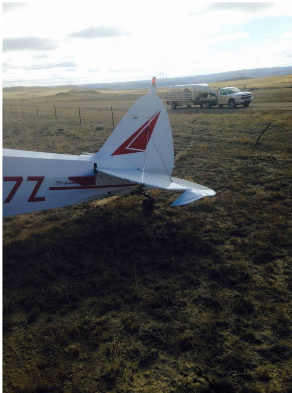
Photo 1 – Substantially Damaged Left Elevator (Photo Courtesy of Operator)
