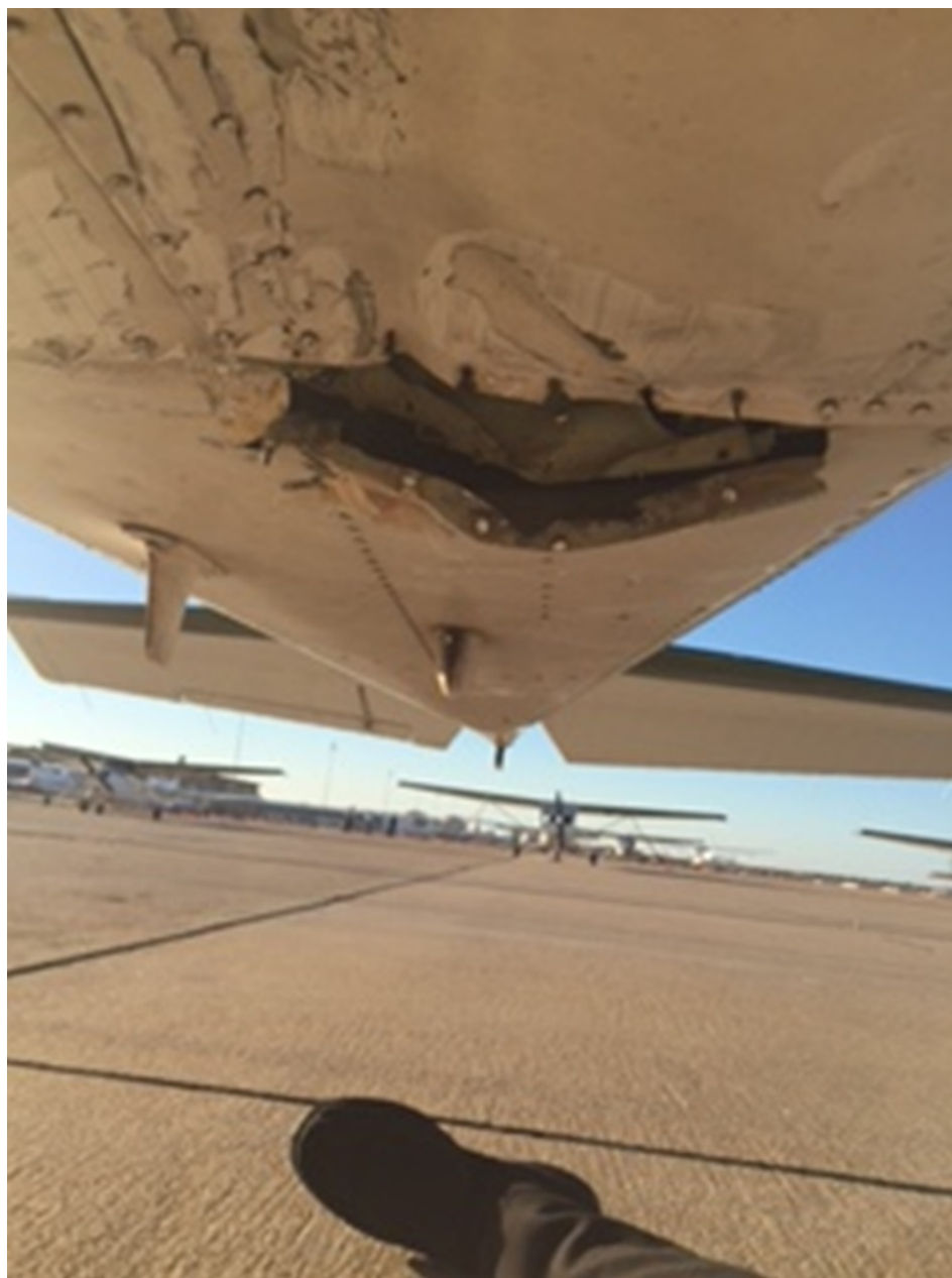
Photo 1 – View of damage to fuselage aft bulkhead (Courtesy of FAA)
