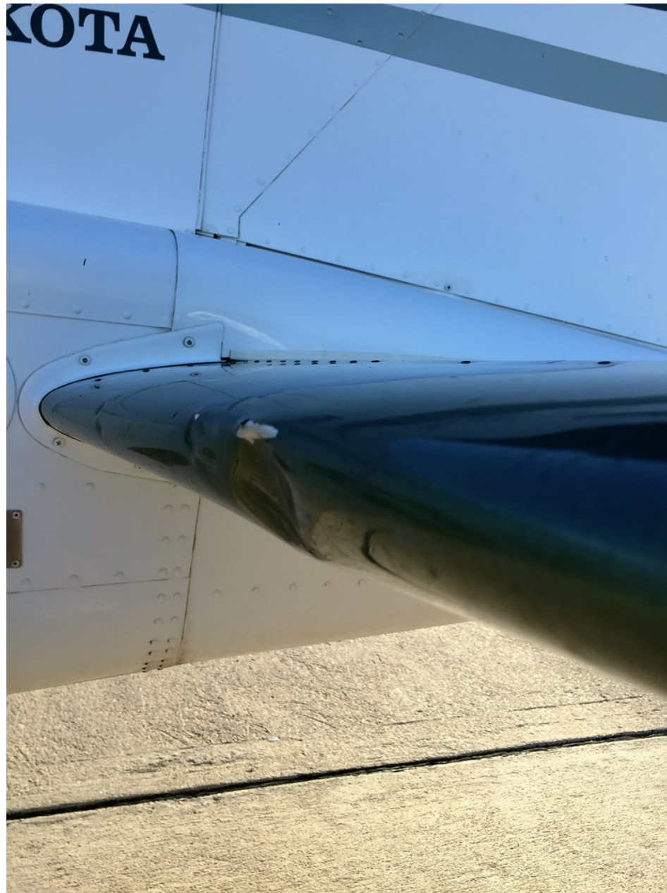
Photo 2 – View of damage to left horizontal stabilizer (Courtesy of FAA)
