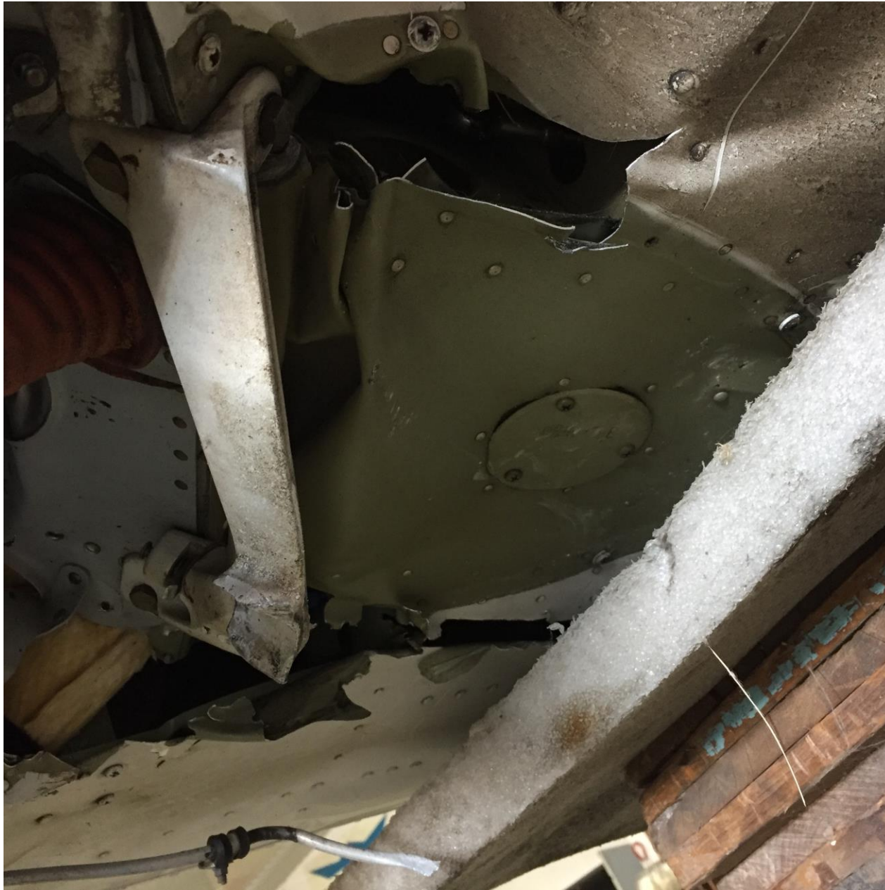
Photo 1 – View of damaged firewall (Photo courtesy of the FAA)
