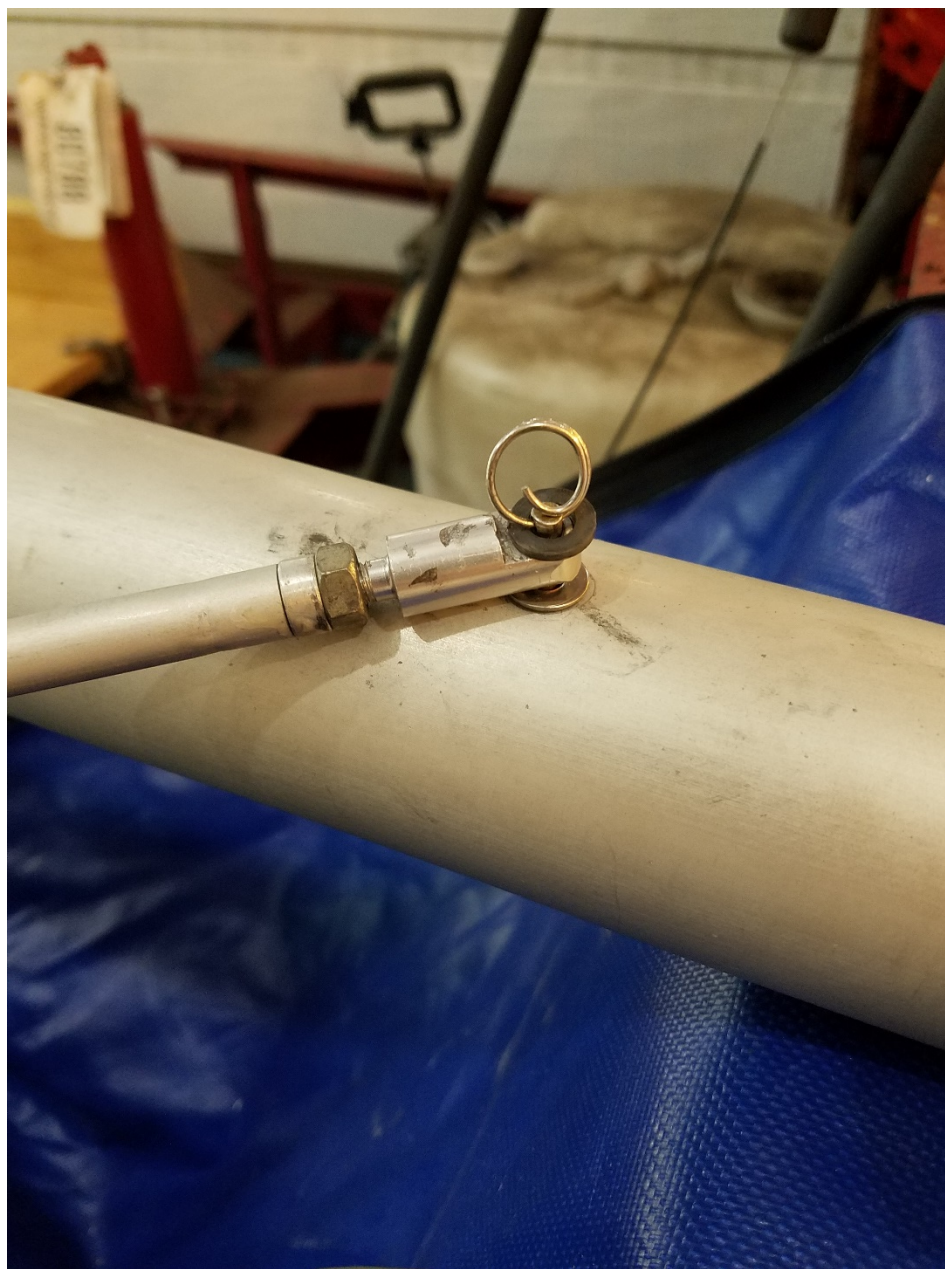
Photo 2 - View of left/good side washout strut and split ring (Courtesy of FAA)
