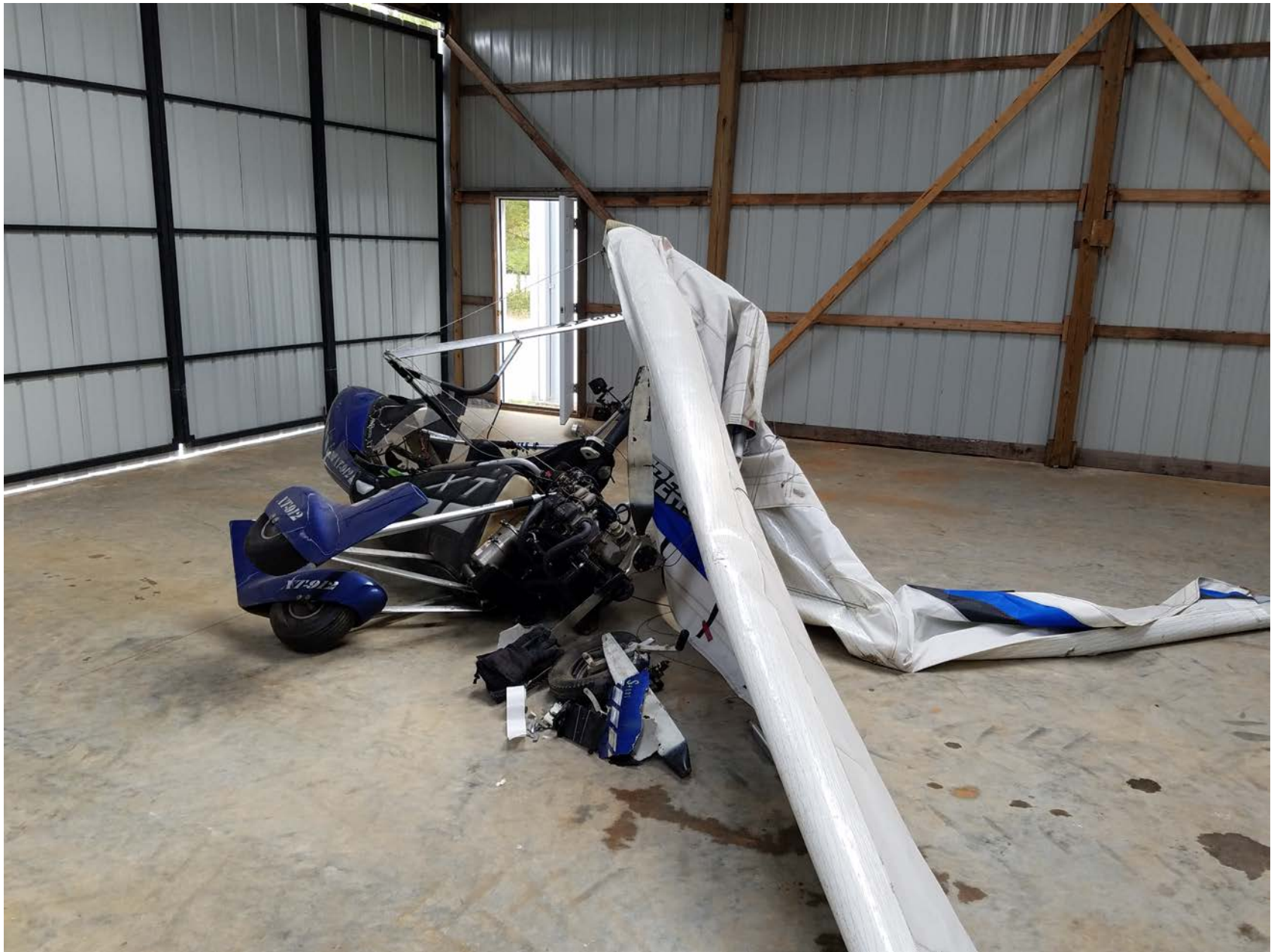
Photo 1 – View of damage to leading edge tube (Courtesy of FAA)
