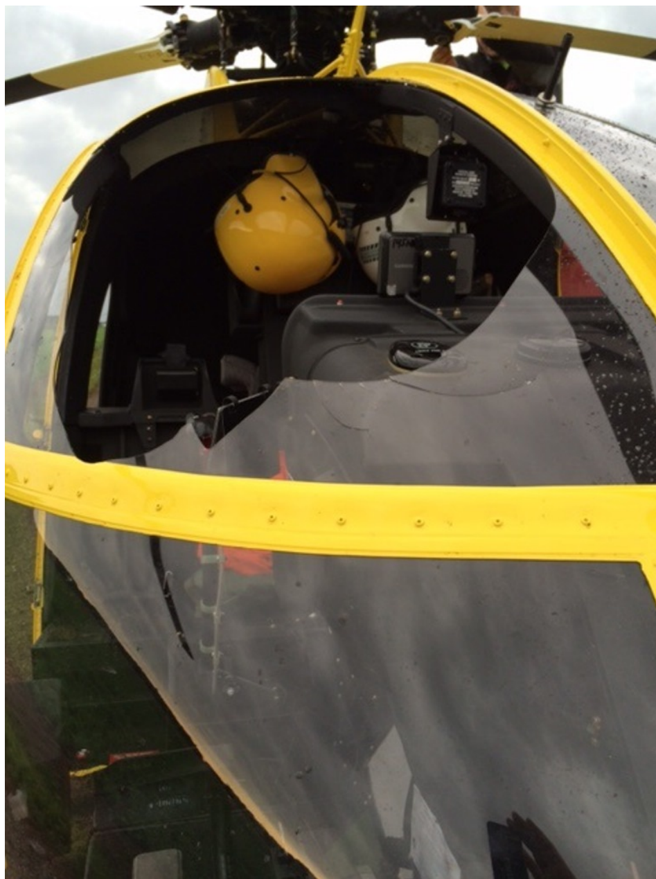
Photo 1 – View of damage to right pilot windscreen (Courtesy of FAA)
