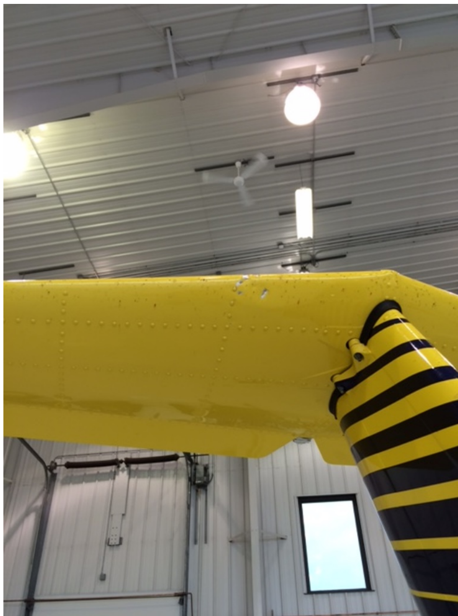
Photo 2 – View of damage to the right side of the horizontal stabilizer (Courtesy of FAA)
