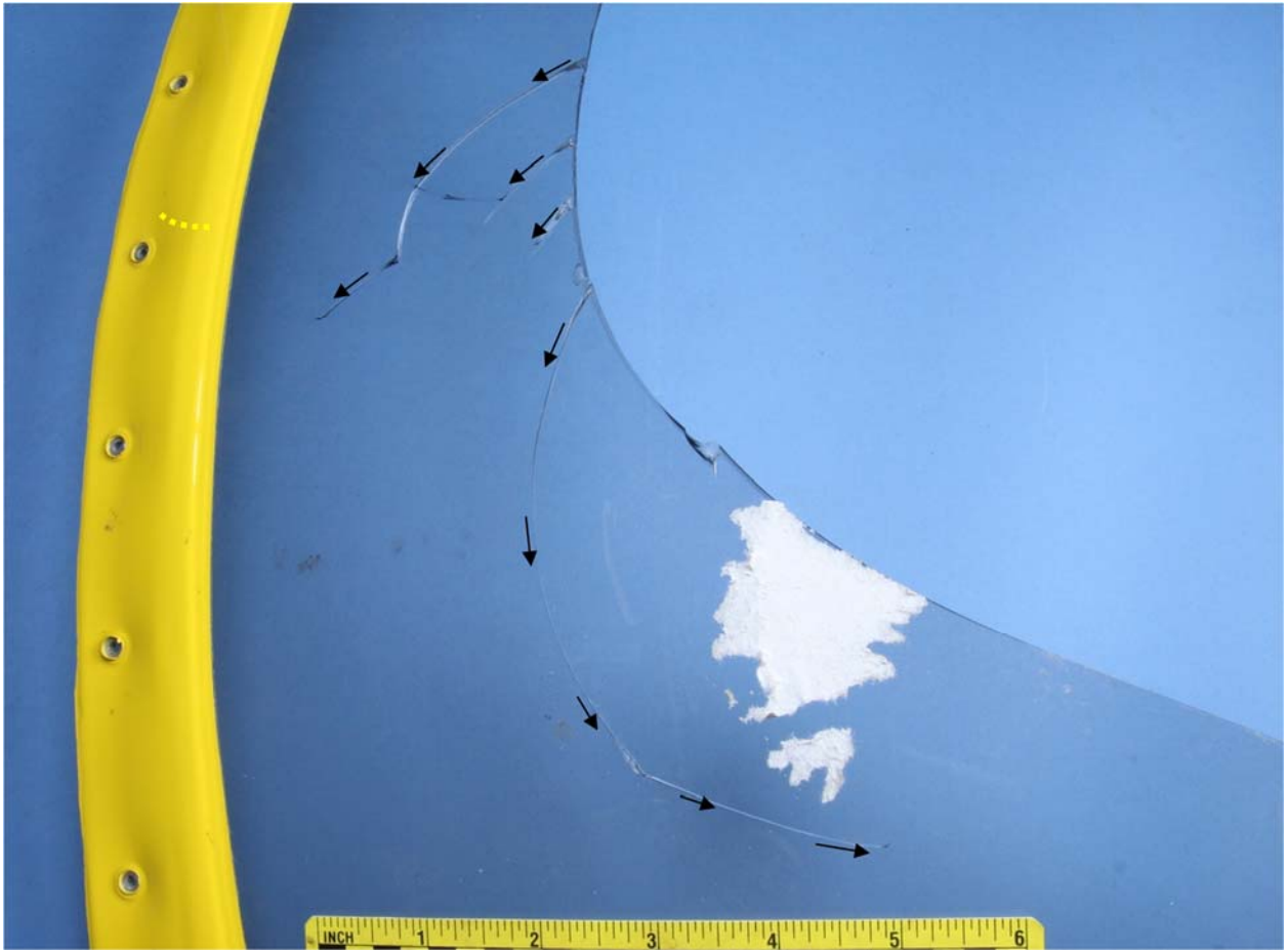
Figure 5: Close-up photo of cracks that had not progressed all the way through the thickness of the windscreen.
