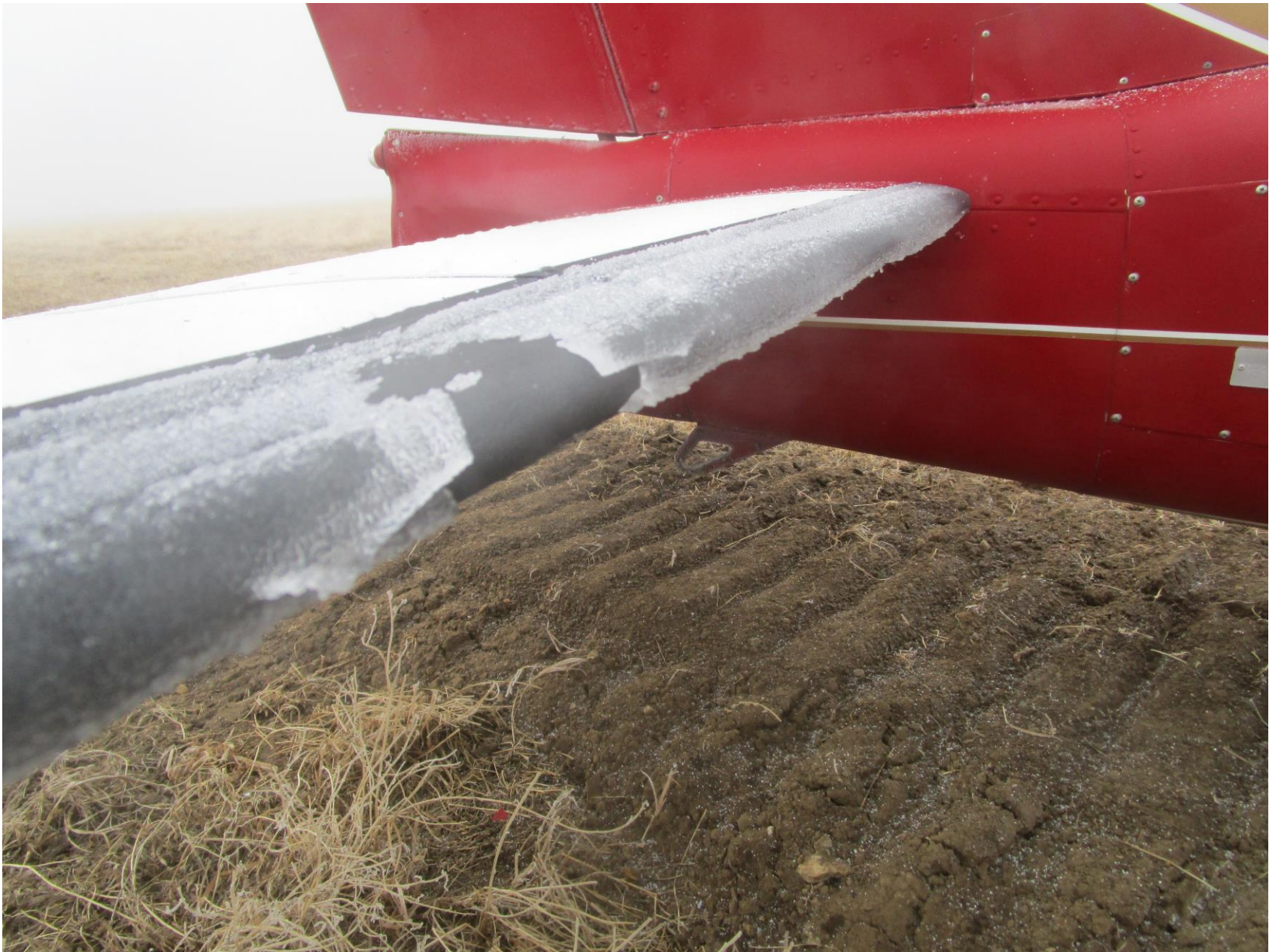
Photo 3 – View of right side horizontal stabilizer with ice accumulation (courtesy of the FAA)
