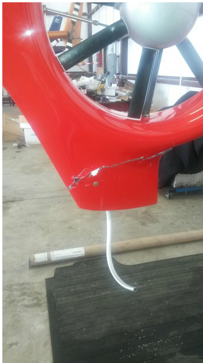
Photo 5 – View of Fenestron housing (courtesy of the operator)
