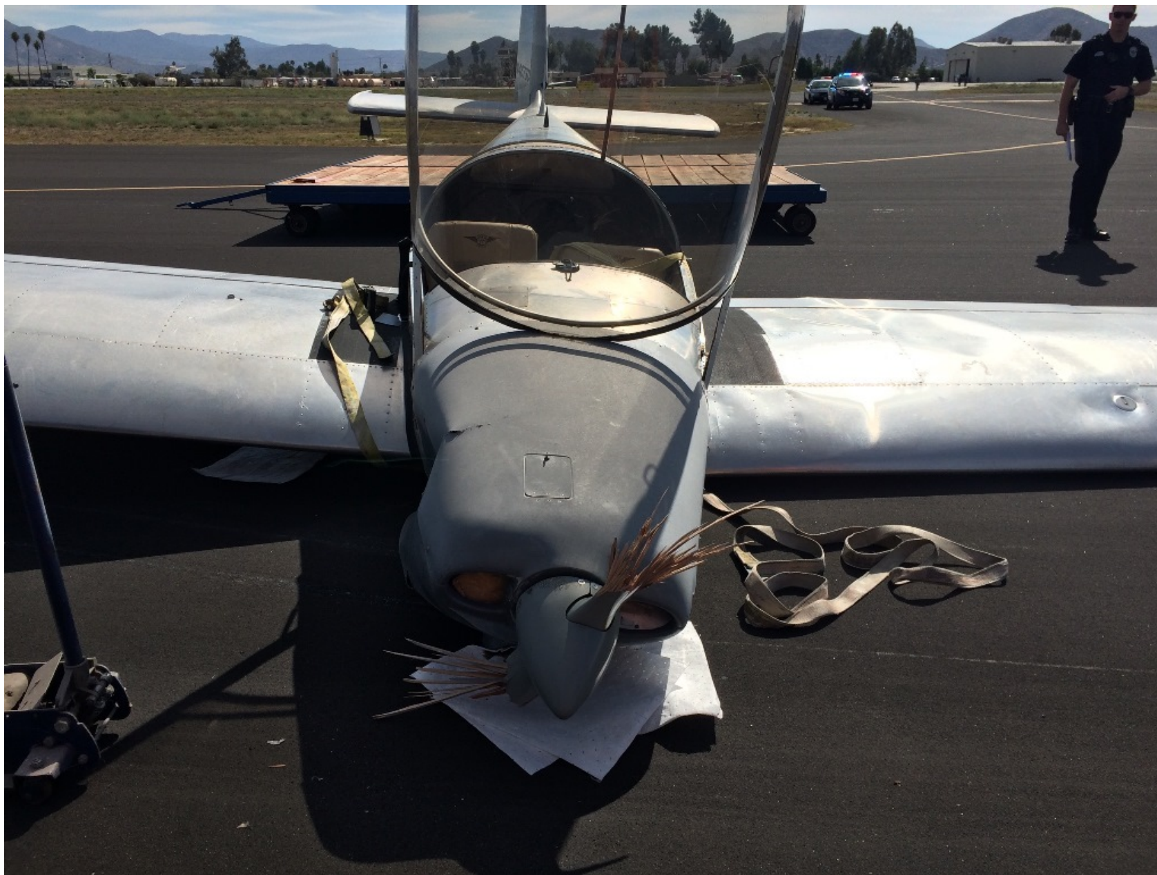
Photo 3 – View of buckling in left wing (Courtesy of FAA)
