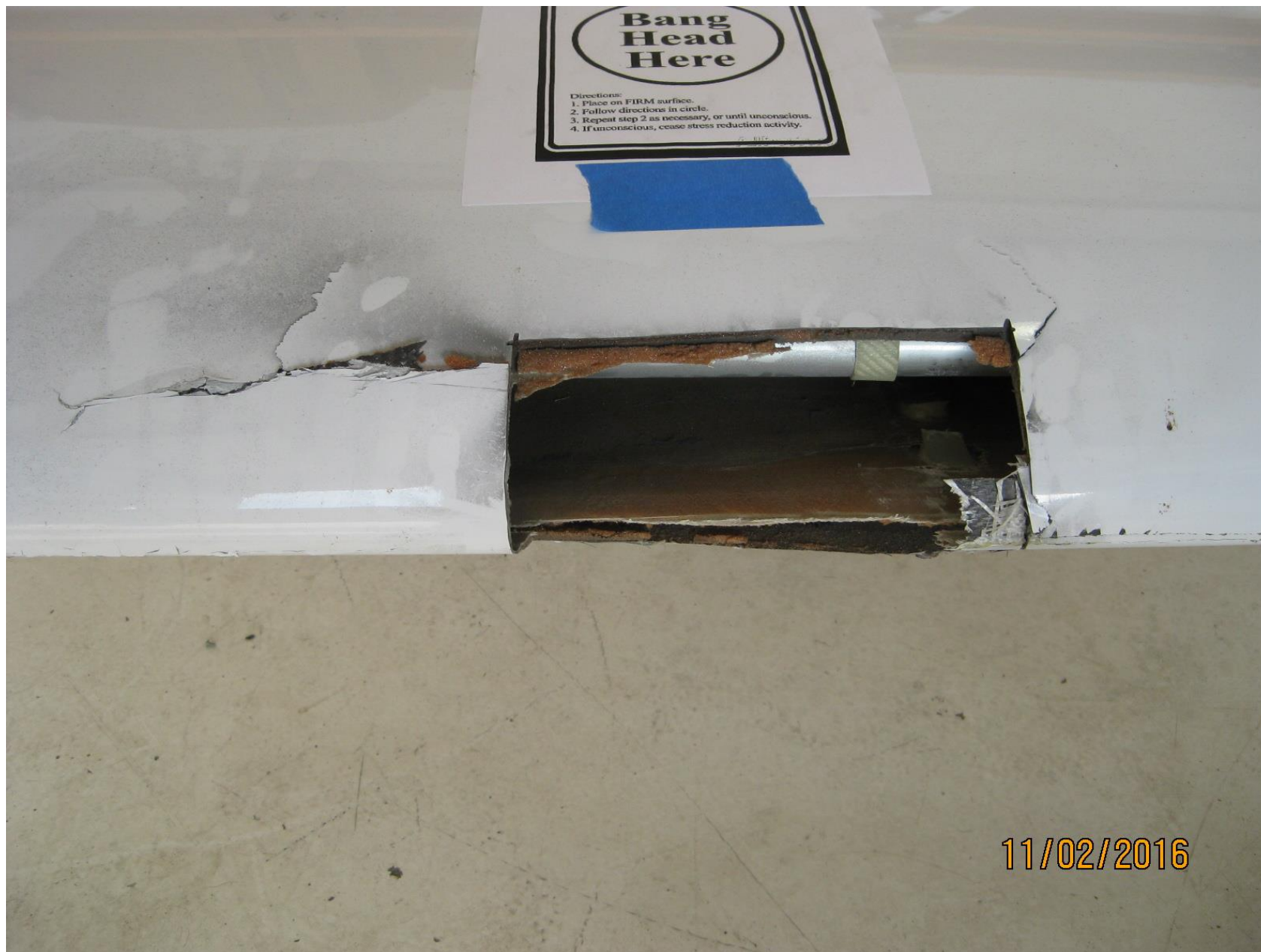
Photo 1 – Substantially Damaged Left Wing (Photo Courtesy of FAA)
