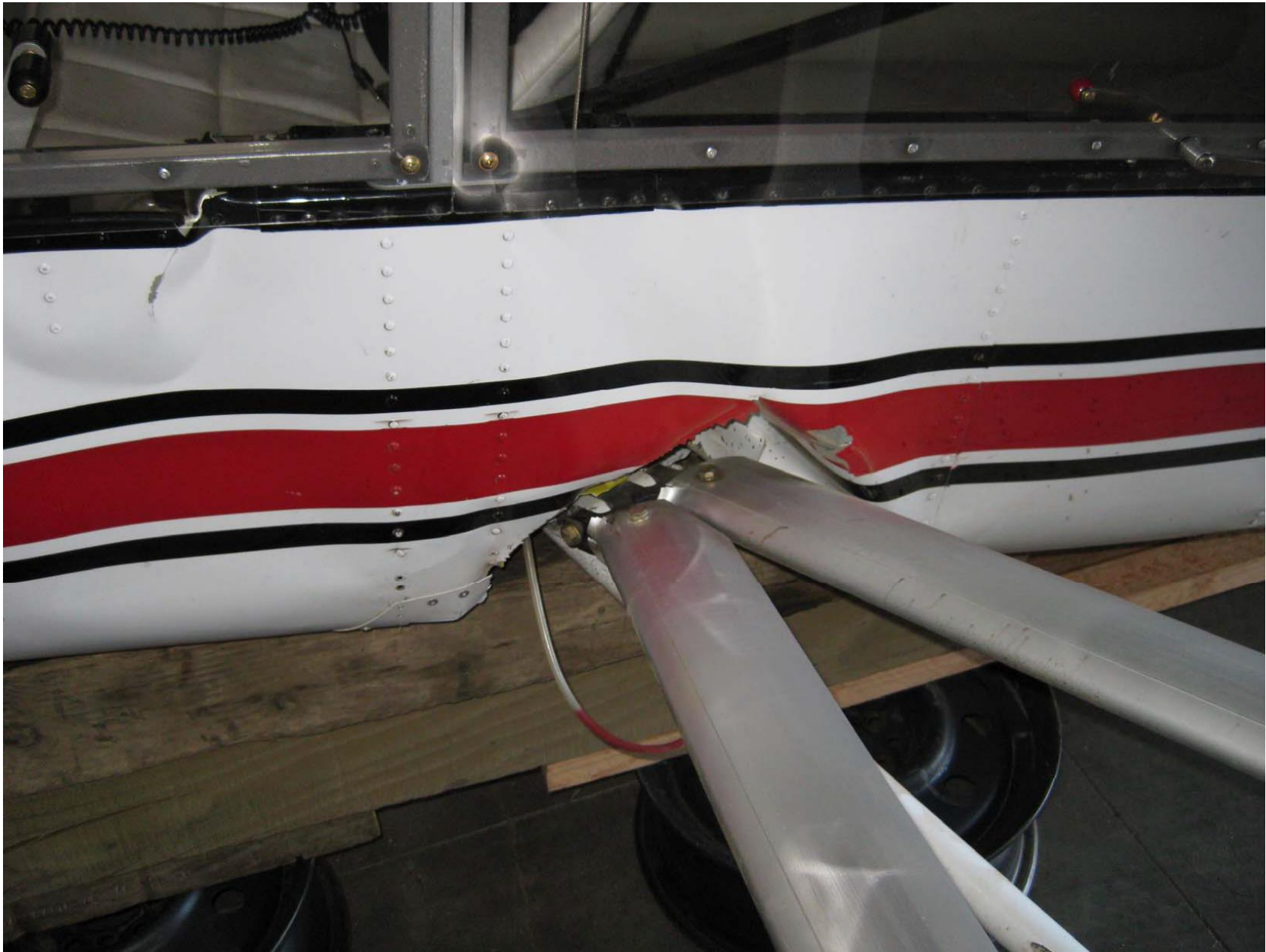
Photo 1 – Damage to spar (Photo courtesy of the FAA)
