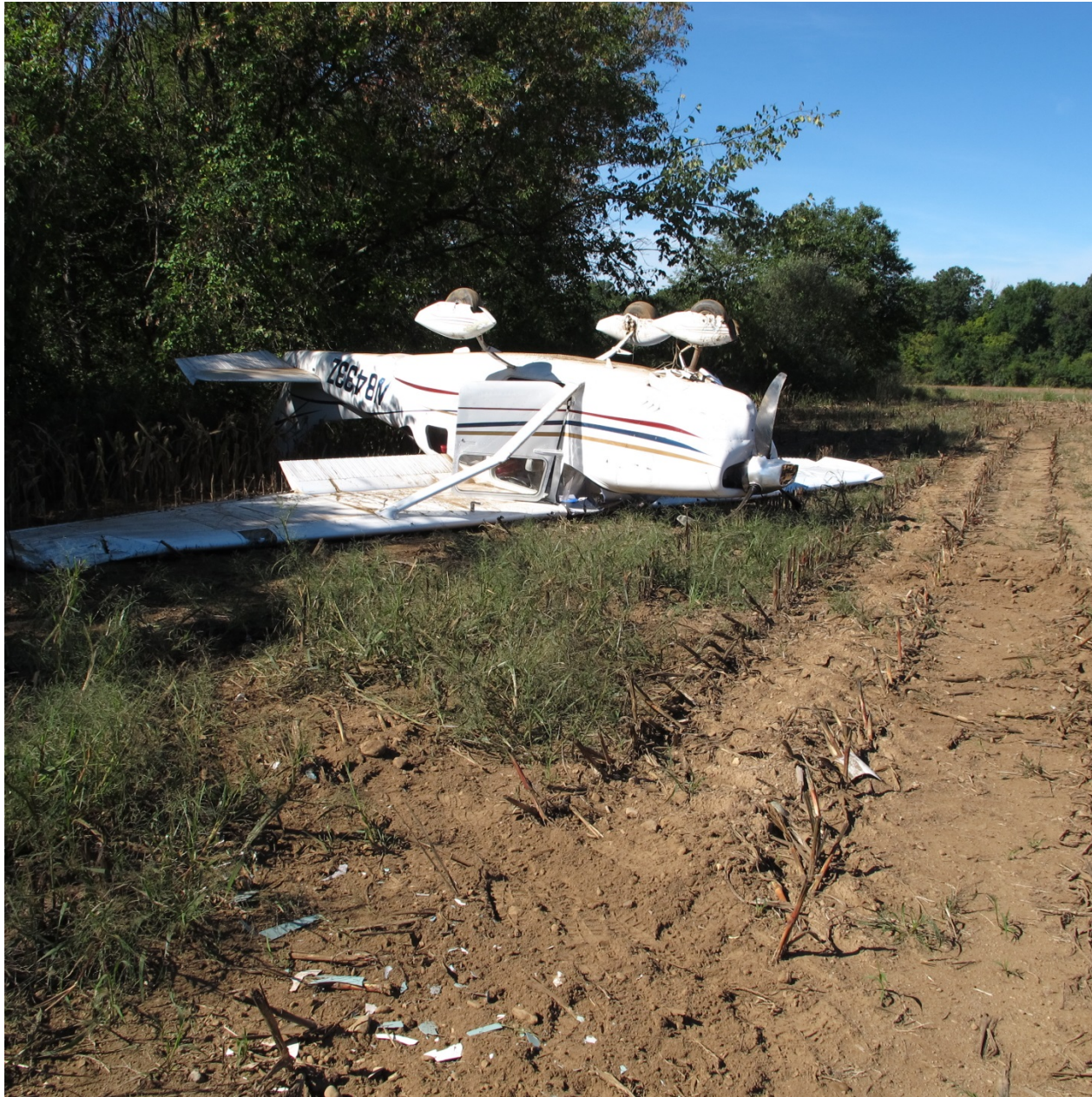
Photo 1 – Airplane Upside Down with Damaged Lift Strut (Photo Courtesy of FAA)
