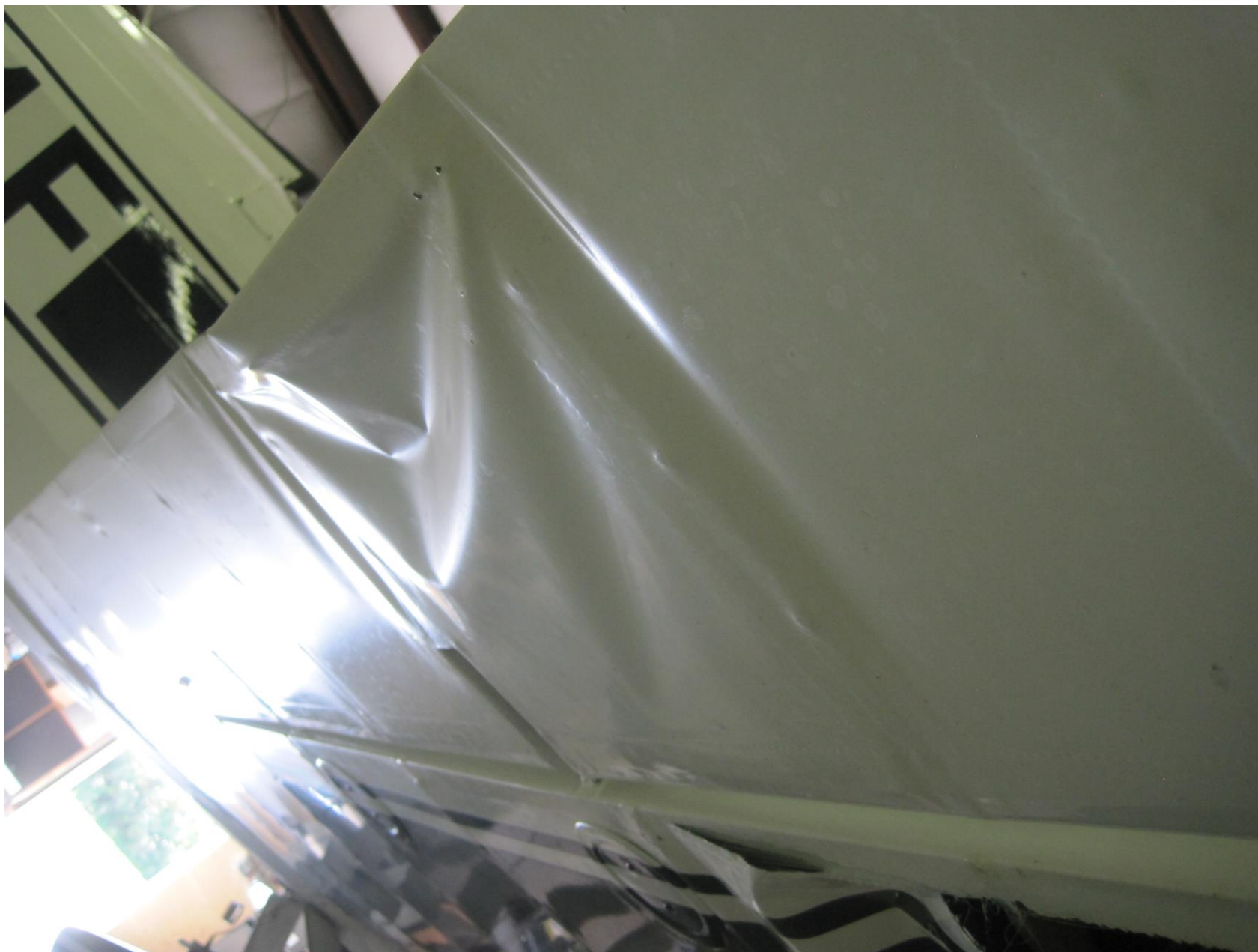
Photo 2 – View of lower right wing aileron damage (photo courtesy of the FAA)
