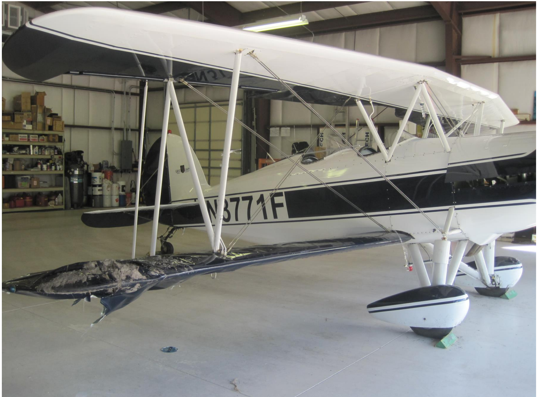
Photo 1 – View of lower right wing damage (photo courtesy of the FAA)
