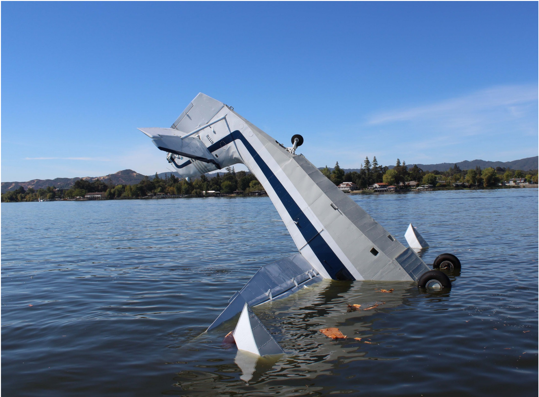
Photo 1 – Nosed Over Airplane in Water (with Landing gear Extended) – (Photo Courtesy of Operator)
