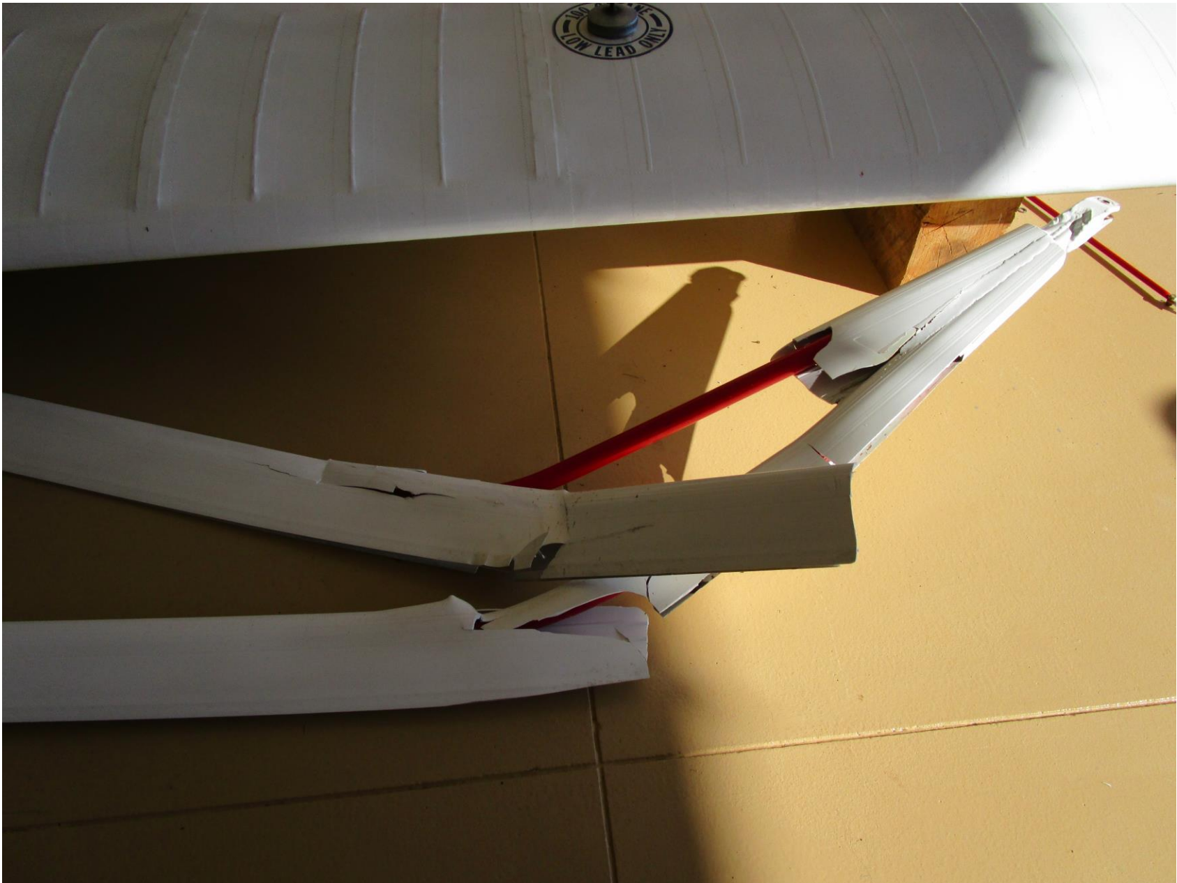
Photo 2 – View of right damaged lift struts (Photo courtesy of the FAA)
